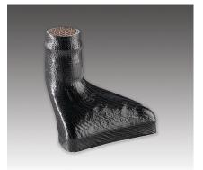
Figure 2: The composite material is then wrapped around the sacrificial tool as shown. Once the part is fully formed and cured, the tool is ready for wash-out.
