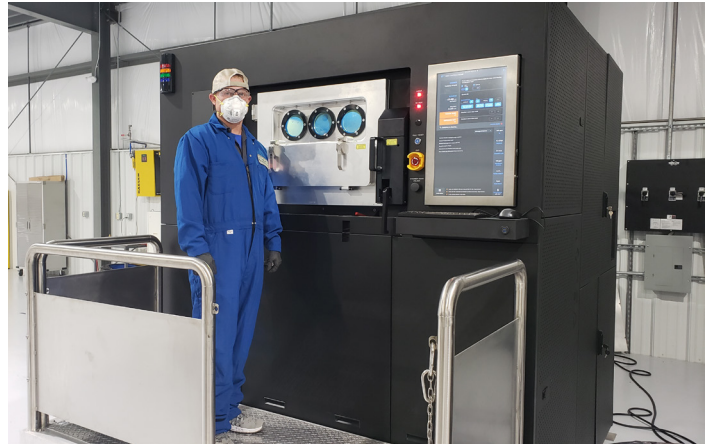
An additive-manufacturing machine operator at Duncan Machine Products (DMP) about to unpack a build on a Sapphire metal 3D-printing system.
