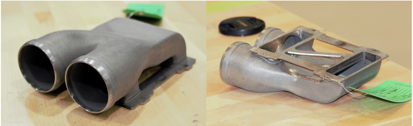
The internal flow passages on XB-1 's VBV fuselage manifolds were printed entirely without support structures, saving material, post-processing time, and labor. Left is the top of the manifold and right is the bottom .
