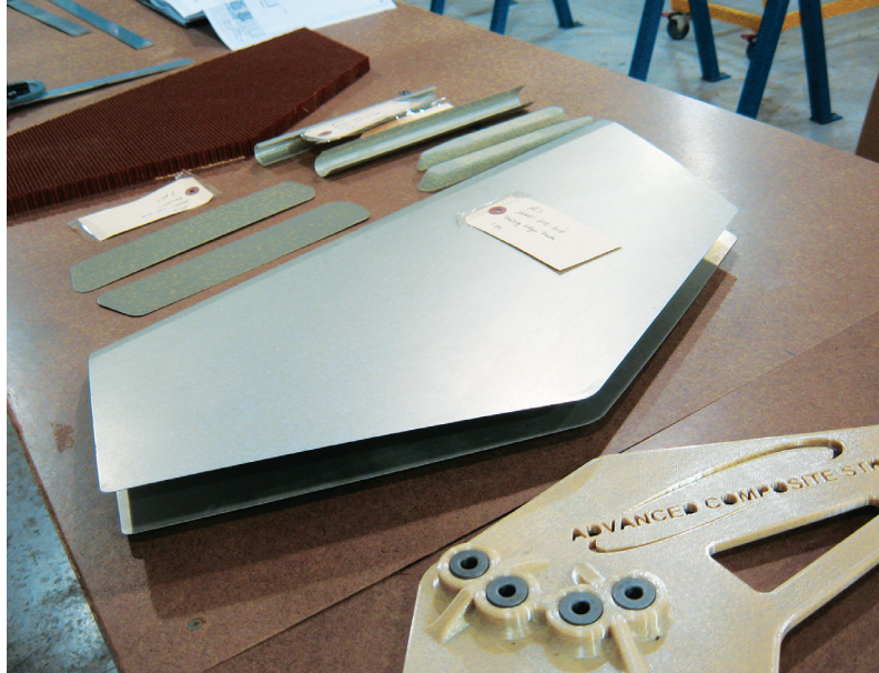
ACS helicopter fin (center) with AM drill guide (front).
