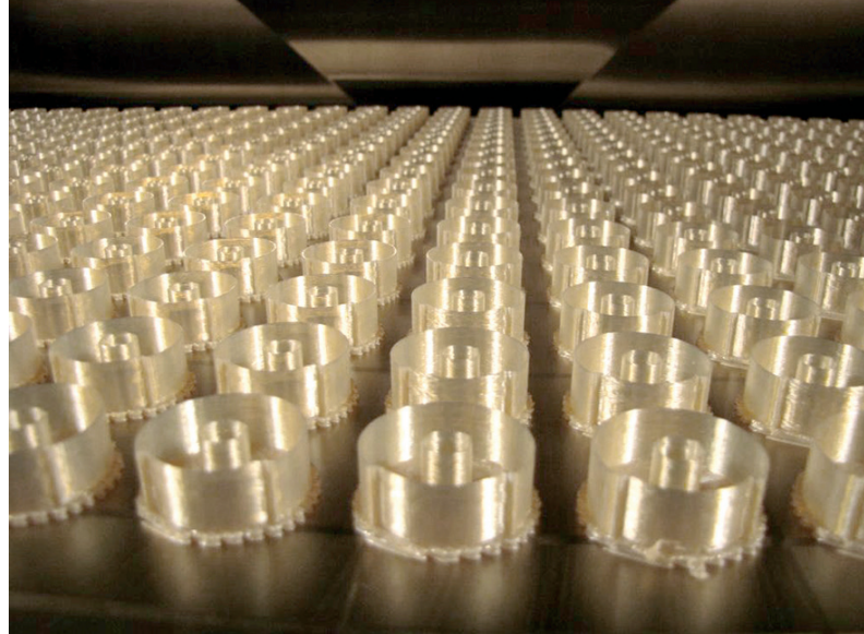
500 toroid housings are produced overnight with an FDM-based Fortus machine.
