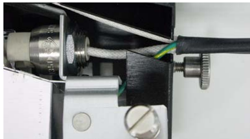
Figure 7-73: Cable position when installing the UV lamp
