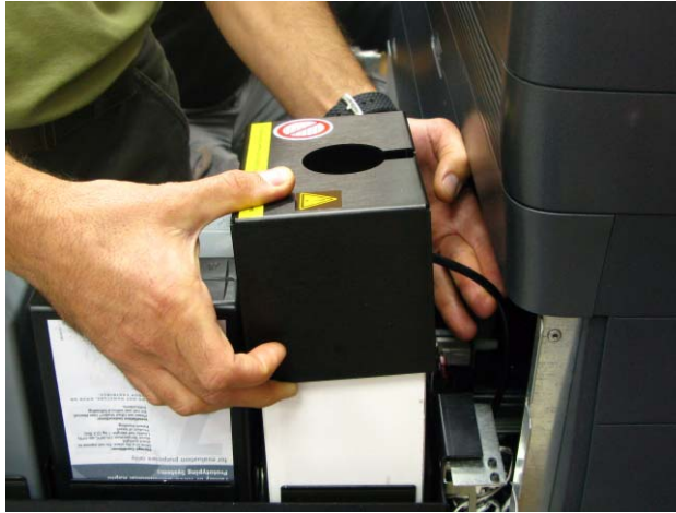
Figure 7-78: Removing the waste-container cover
