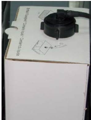
Figure 7-79: Waste container with drain tube attached
