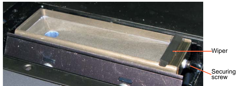
Figure 7-30: Wiper and excess-material drain
