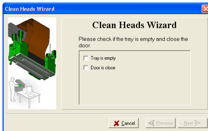
Figure 7-20: Head cleaning procedure—wizard screen
