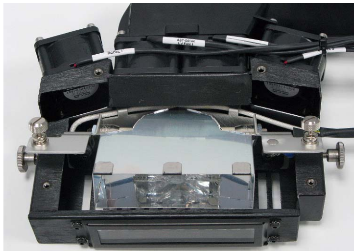
Figure 7-72: Removing the UV reflector from the UV assembly
