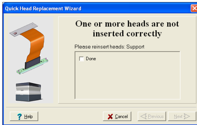
Figure 7-53: Incorrect-installation screen, showing which head(s) to re-insert
