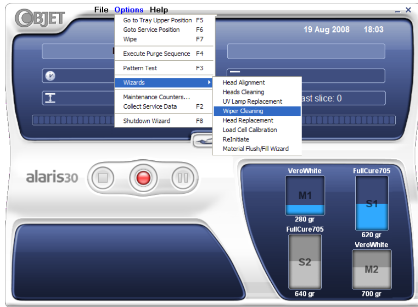
Figure 7-27: Starting the Wiper Cleaning wizard
