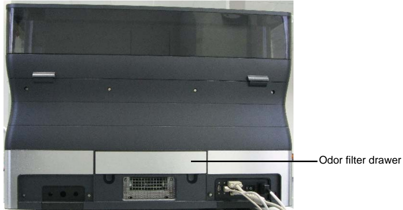
Figure 7-64: Rear of the Alaris30 printer
