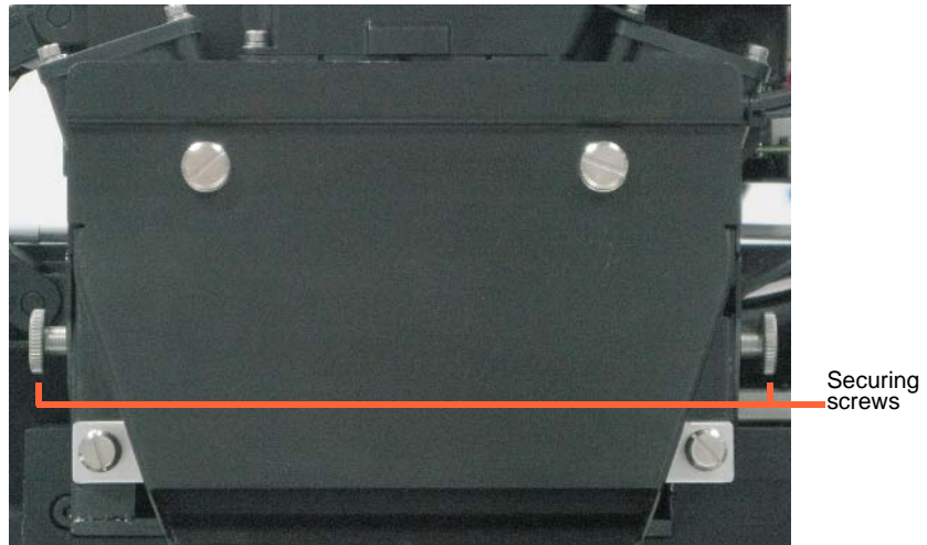
Figure 7-35: UV-lamp-assembly securing screws
