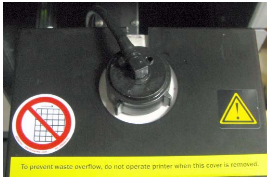
Figure 7-80: Fireproof cover installed over the waste container
