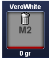
Figure 7-6: Empty cartridge indicator
