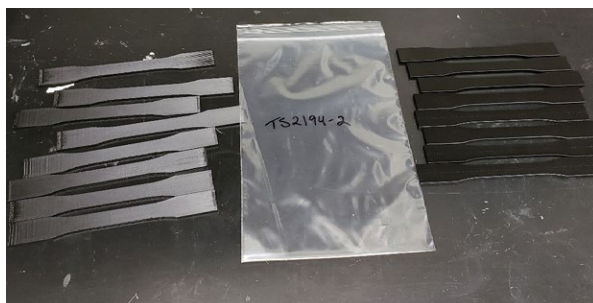
Figure 2. Samples after exposure to Skydrol.
