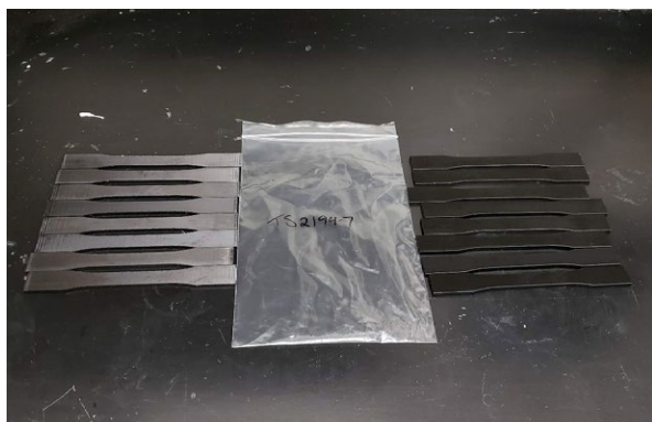
Figure 7. Samples after exposure to Jet A.
