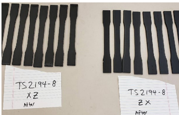
Figure 8. Samples after exposure to 30% nitric acid.
