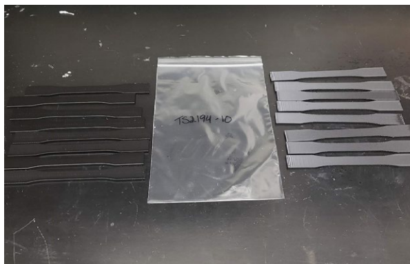
Figure 10. Samples after exposure to 60% sodium hydroxide.
