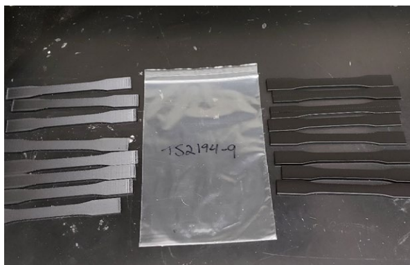
Figure 9. Samples after exposure to 30% sulfuric acid.
