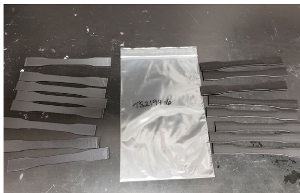
Figure 6. Samples after exposure to toluene.
