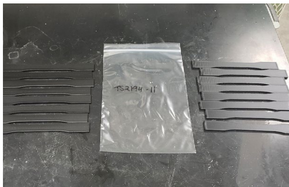
Figure 11. Samples after exposure to concentrated ammonium hydroxide.
