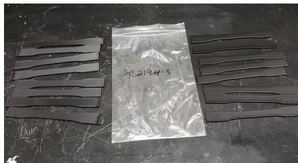
Figure 3. Samples after exposure to MEK.
