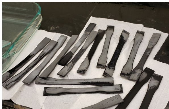
Figure 4. Samples after exposure to DCM.
