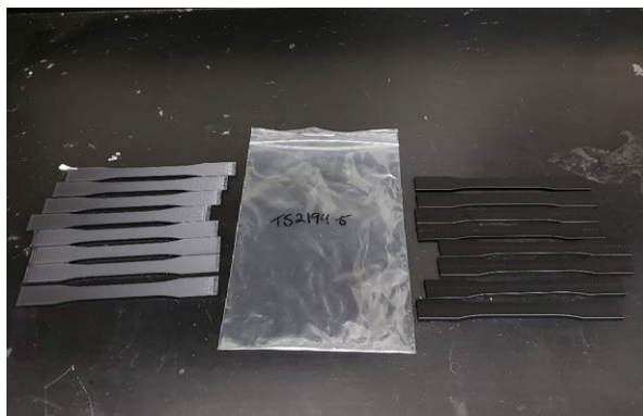
Figure 5. Samples after exposure to ethyl acetate.
