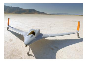
Final 3D printed jet-powered aircraft.
