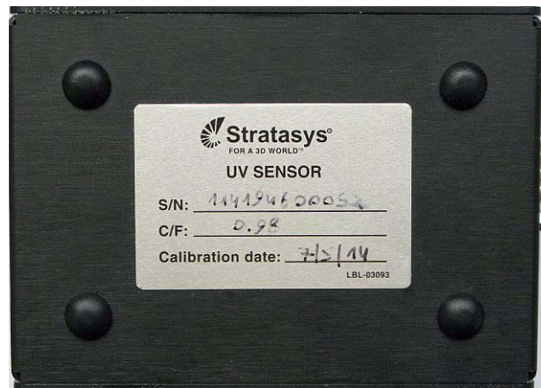
Figure 6-77: Label on the bottom of the UV sensor
