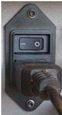
Figure 6-2: Main power switch and cable
