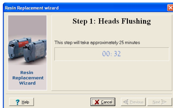
Figure 7-12: Resin replacement (long cycle): flushing heads with cleanser
