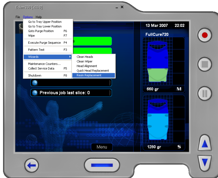
Figure 7-7: Starting the Resin Replacement wizard from the Options menu
