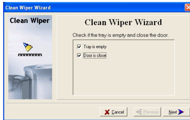
Figure 7-24:Wiper Cleaning procedure—step 4
