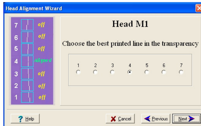
Figure 7-32: Head alignment screen
