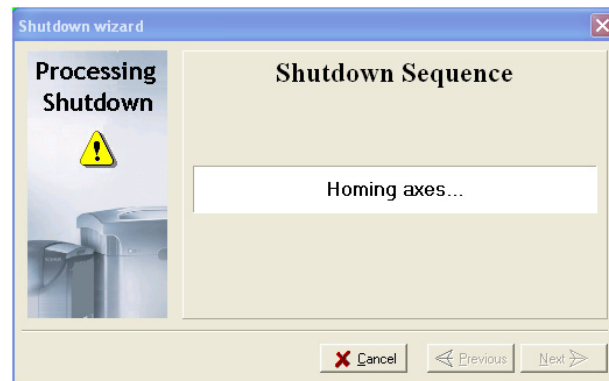
Figure 7-16:Shutdown dialog box, showing first step in the procedure
