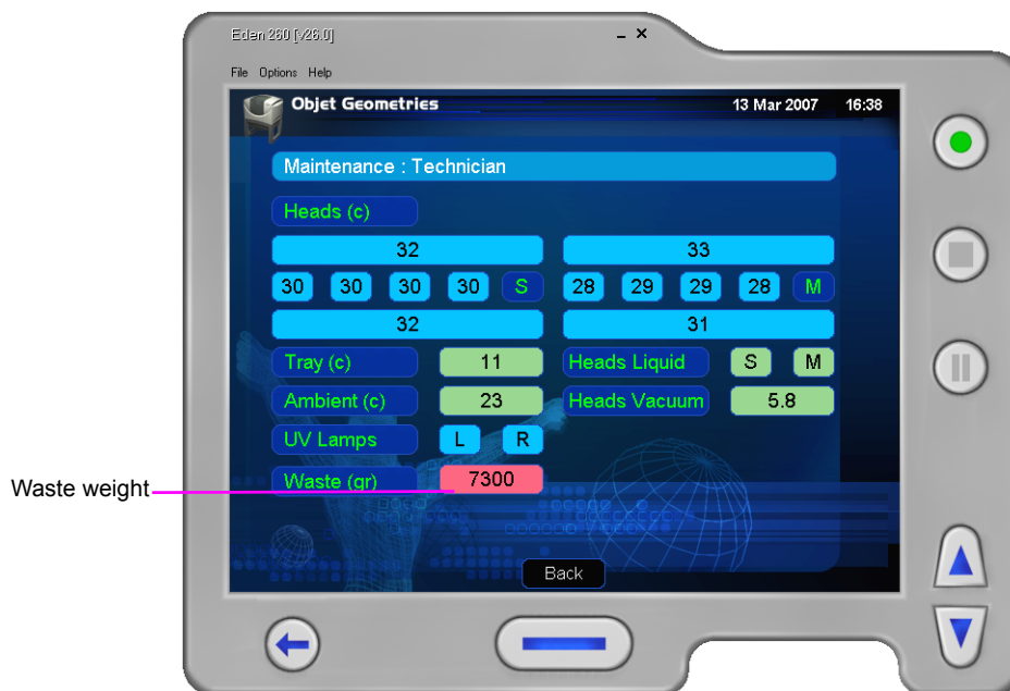
Figure 7-67: Eden printer interface, showing waste weight (red background indicates operator alert)
