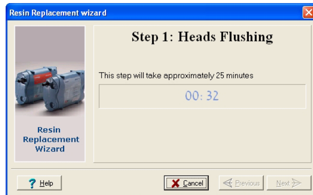
Figure 7-11: Resin replacement (long cycle): flushing heads with cleanser
