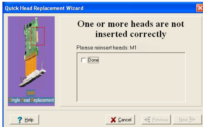
Figure 7-51: Incorrect-installation screen, showing which head(s) to re-insert
