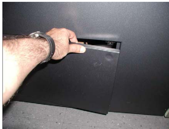
Figure 7-4: Accessing the waste container
