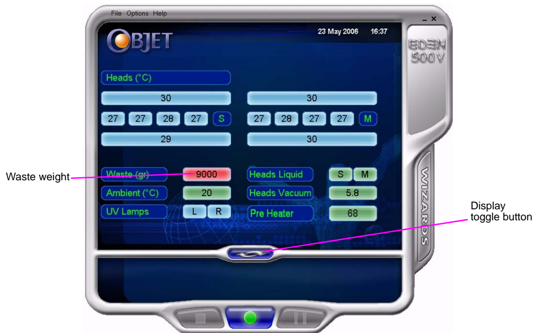
Figure 7-3: Eden printer interface, showing waste weight (red background indicates operator alert)
