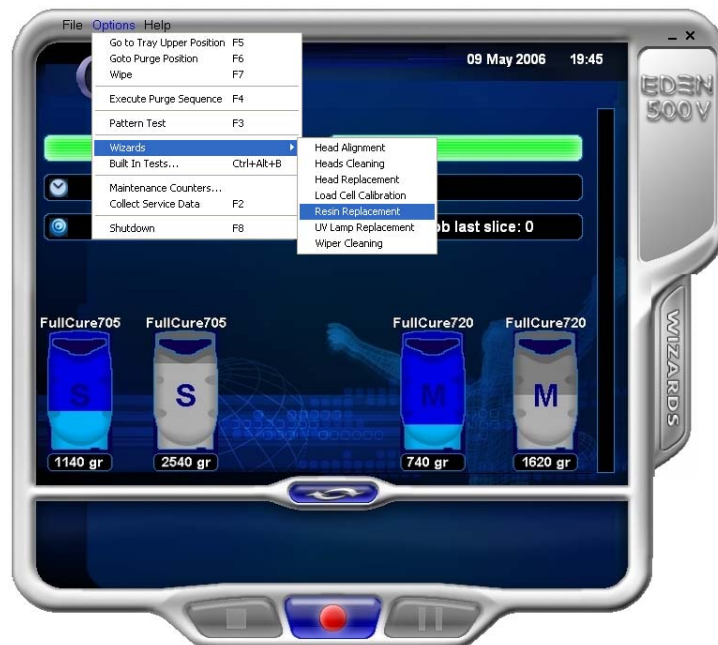
Figure 7-9: Starting the Resin Replacement wizard from the Options menu
