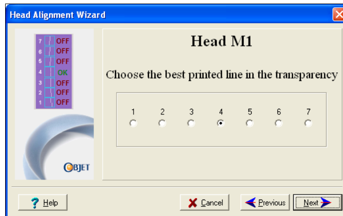
Figure 7-32: Head alignment screen
