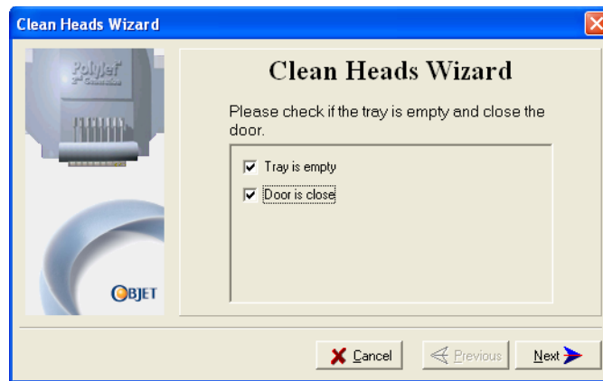
Figure 7-19: Head cleaning procedure—wizard screen
