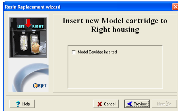
Figure 7-14: Prompt to insert new right-hand model cartridge
