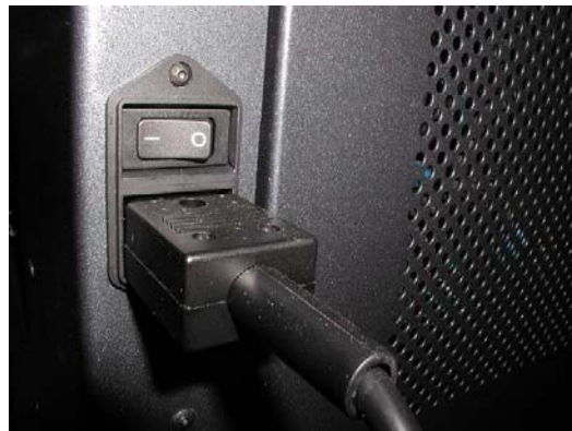
Figure 7-2: Main power cable and switch
