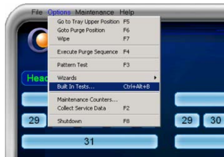
Figure 7-1: Selecting Built-In Tests from the Options Menu
