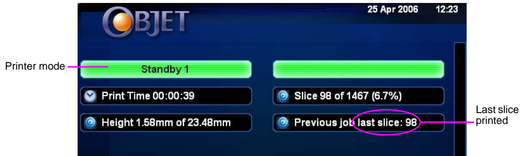
Figure 7-6: Eden printer interface after interrupted printing
