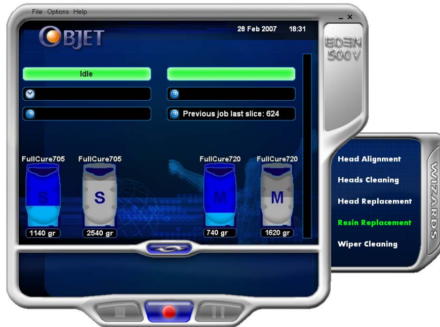
Figure 7-8: Starting the Resin Replacement wizard from the Wizards tab
