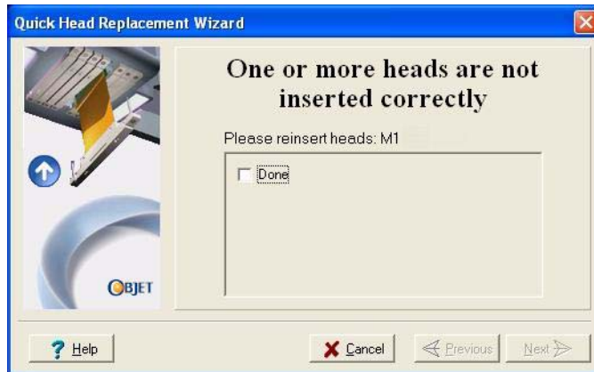
Figure 7-50: Incorrect-installation screen, showing which head(s) to re-insert
