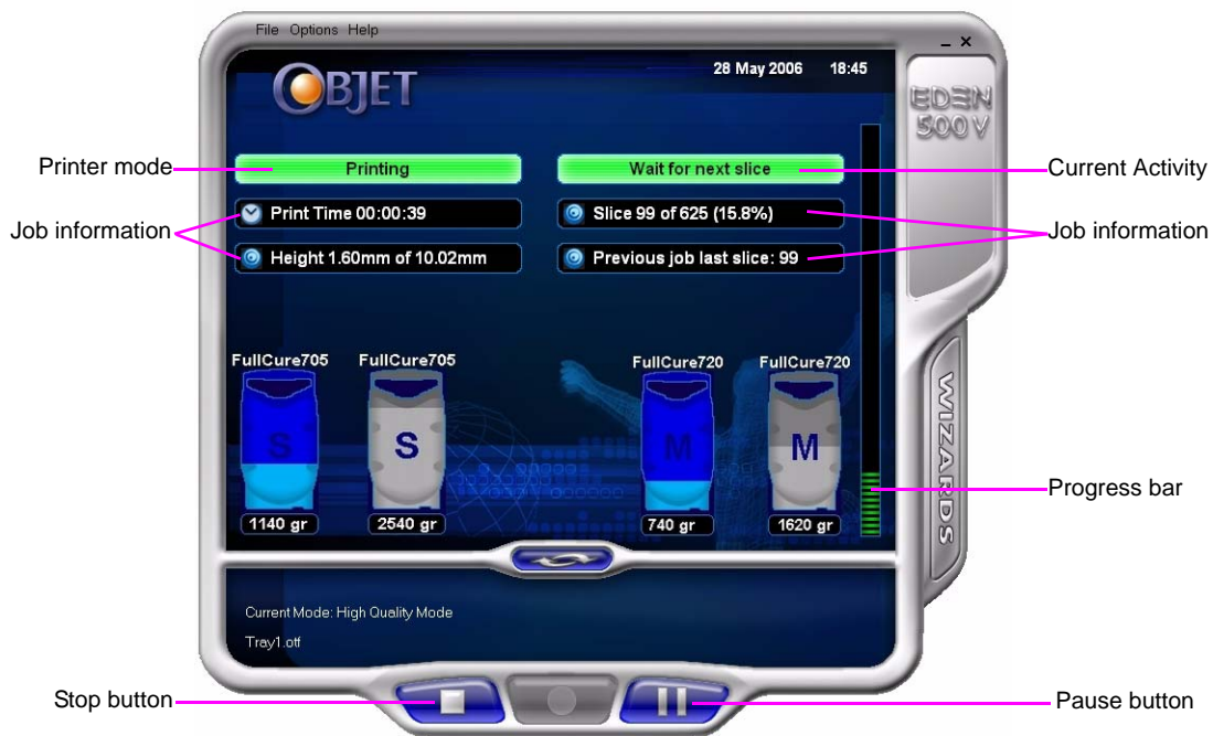
Figure 7-5: Eden printer interface during printing
