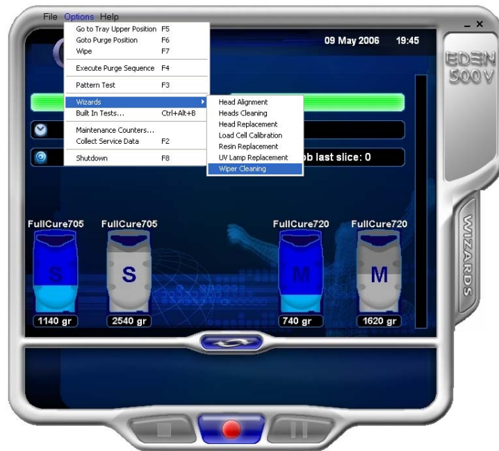
Figure 7-25: Starting the Wiper Cleaning wizard
