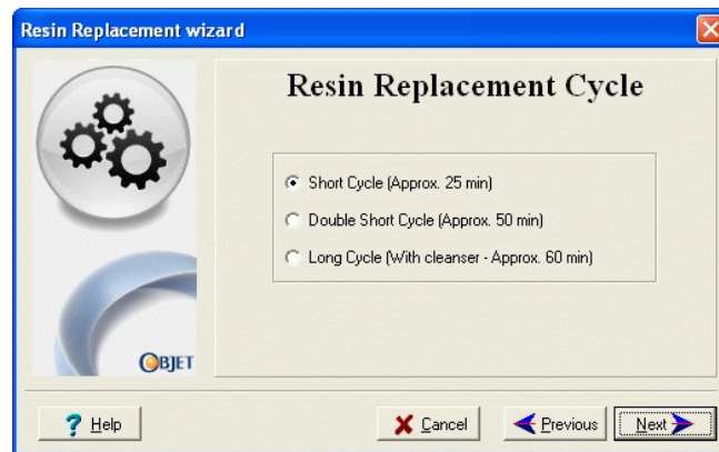
Figure 7-12: Resin Replacement Cycle screen
