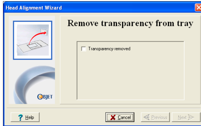
Figure 7-29: Head Alignment wizard—steps 8–10
