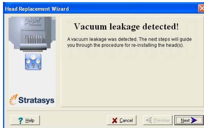
Figure 6-73: Vacuum-leakage warning screen
