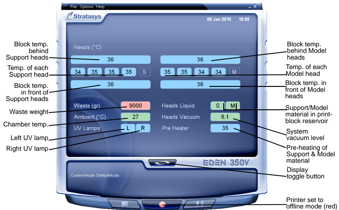
Figure 6-4: Printer indicators
