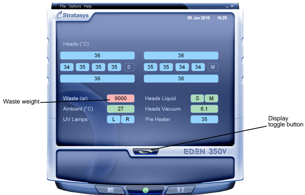
Figure 6-107: Printer interface, showing waste weight (red background indicates operator alert)
