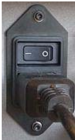
Figure 6-2: Main power switch and cable
