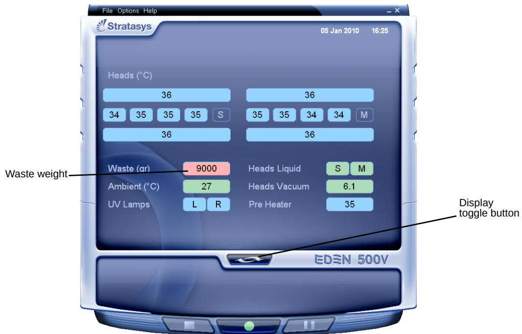
Figure 6-105: Printer interface, showing waste weight (red background indicates operator alert)
