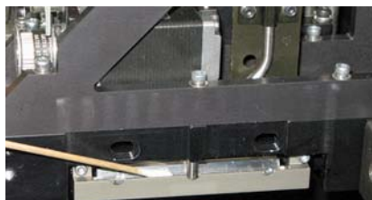
Figure 6-37: Cleaning the roller waste collector
