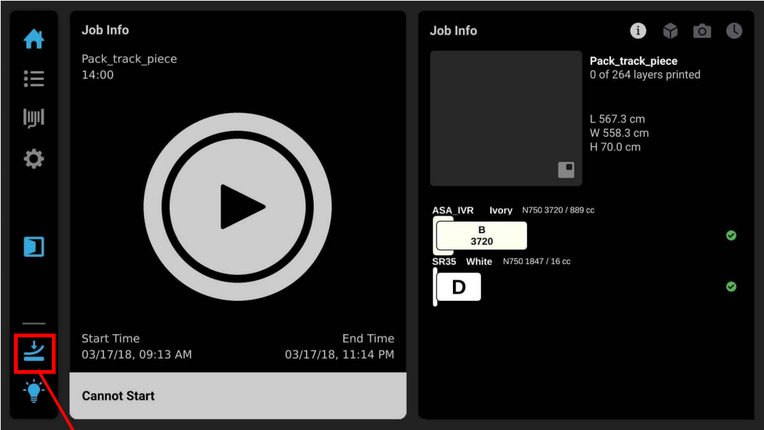
Figure 136: Vacuum enabled, but not achieved
