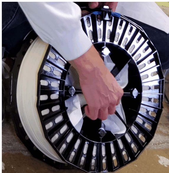
Figure 165: Removing Desiccant Bags
