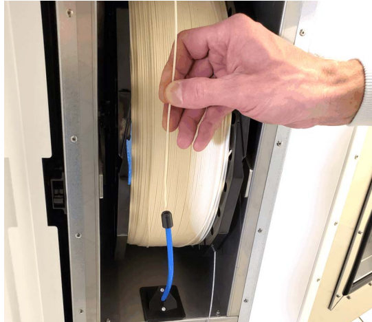
Figure 169: Feeding the Filament into the Guide Tube
