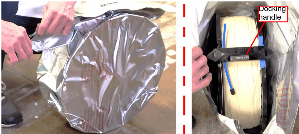
Figure 164: Inside the Material Spool Bag
