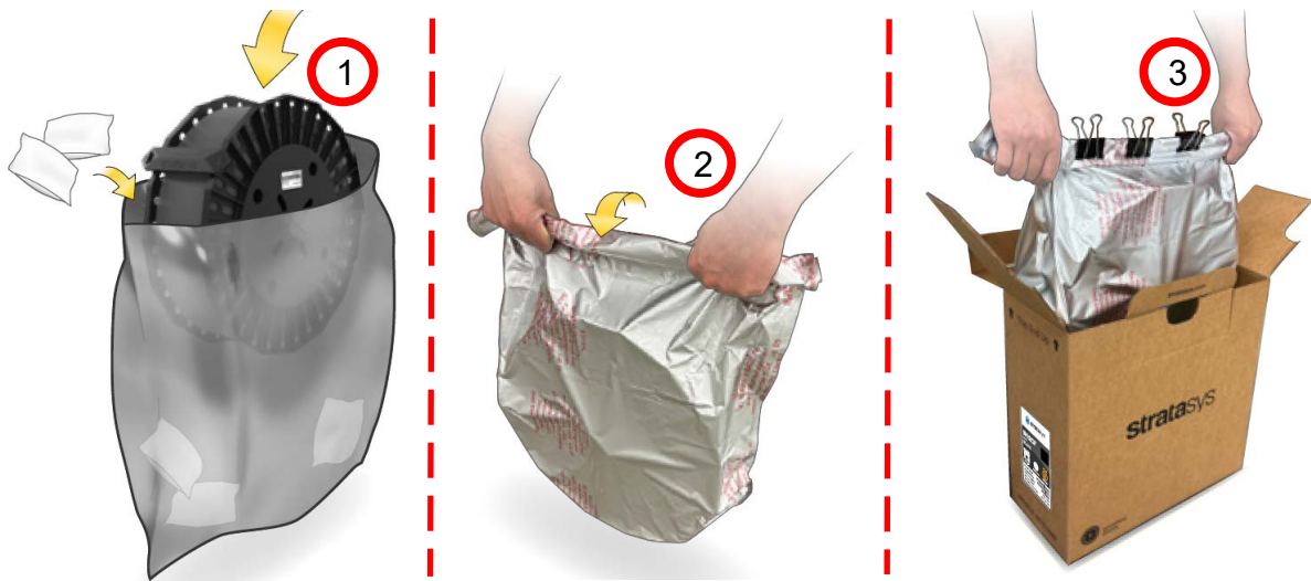
Figure 187: Resealing the Spool Bag Option 1: Roll and Clip the Bag Opening
