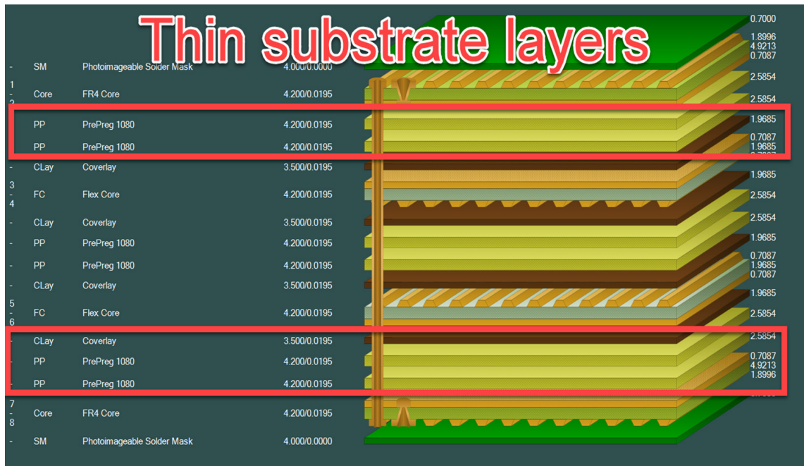
Real thicknesses of substrate layers
