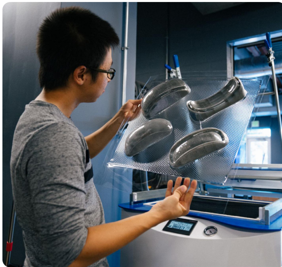
Thermoforming is a common method for producing plastic packaging. This packaging was thermoformed on a 3D printed mold.
