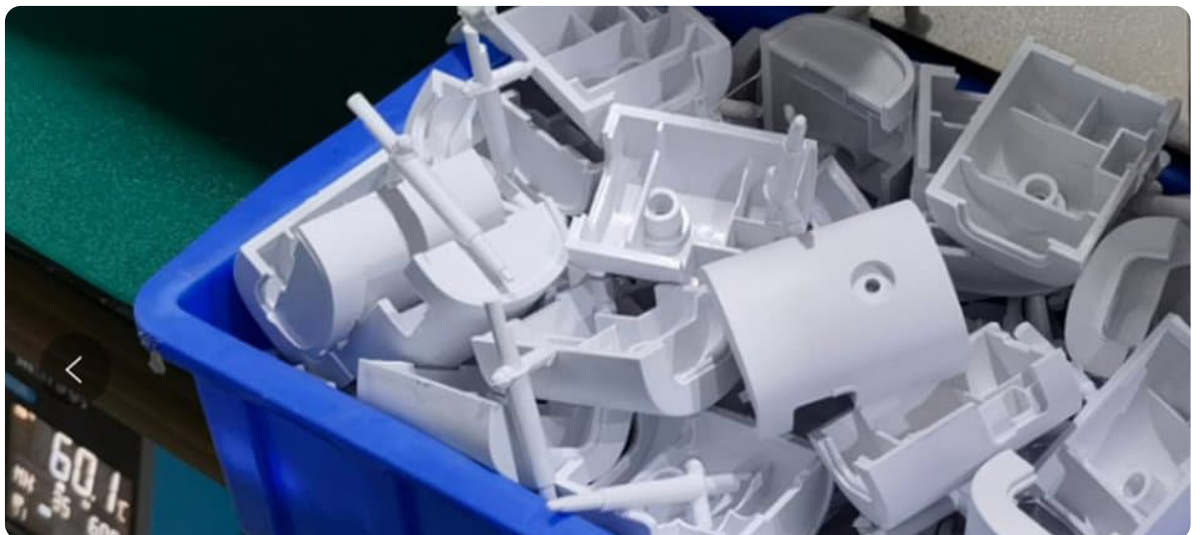
ABS control box housings injection molded using 3D printed molds.
