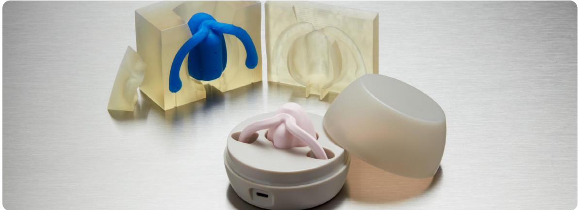
Dame Products employs silicone insert molding to encapsulate internal hardware for customer beta prototypes.
