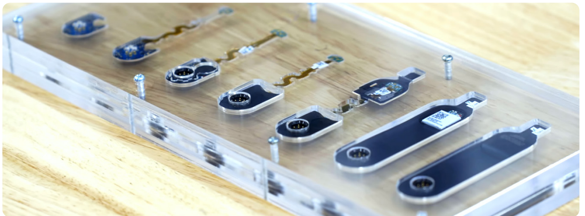
Google's ATAP team used 3D printed stand-ins, or surrogate parts instead of overmolded electronic sub-assemblies for the initial tool tuning at the factory
