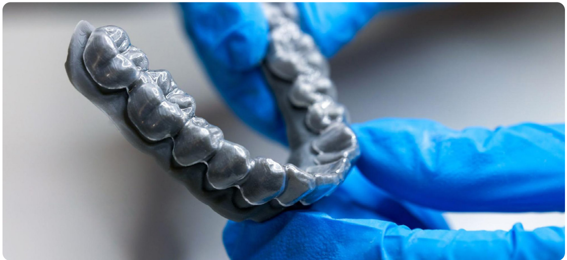
Vacuum forming and pressure forming over 3D printed models are the go-to methods for producing clear aligners in orthodontics.
