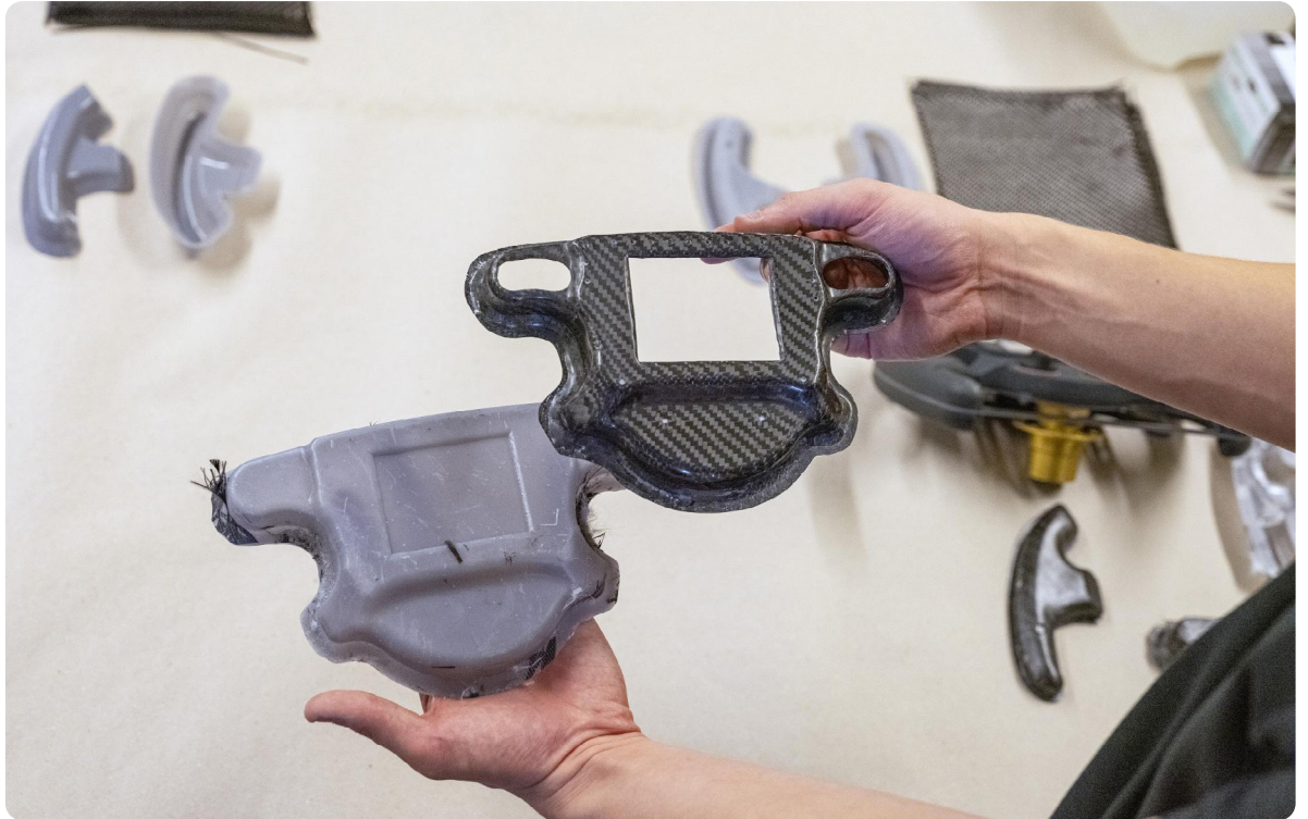
The 3D printed mold and the demolded carbon fiber part for the steering wheel front housing.
