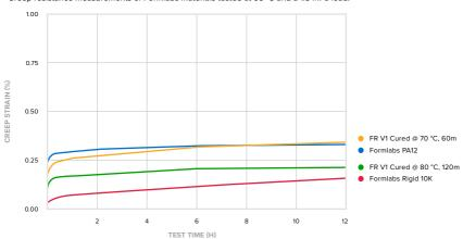
Formlabs Flame Retardant Resin parts have high creep resistance. Post-curing Flame Retardant Resin samples at 80 °C for 120 minutes shows improved creep resistance compared to post-curing at 70 °C for 60 minutes. Flame Retardant Resin samples post-cured at 80 °C and 120 minutes is slightly lower in creep resistance than Rigid 10K Resin samples. Flame Retardant Resin samples post-cured at 70 °C and 60 minutes showed similar creep behavior as Formlabs Nylon 12 SLS Powder.
