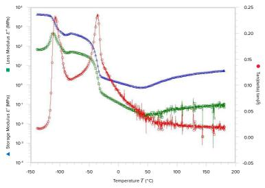
A DMA curve from -150 deg C to 180 °C at 3 °C/min is shown. A glass transition is observed at -107 °C, and a crystalline melting transition is observed at -37 °C followed by a rubbery plateau to the conclusion of the test at 180 °C.
