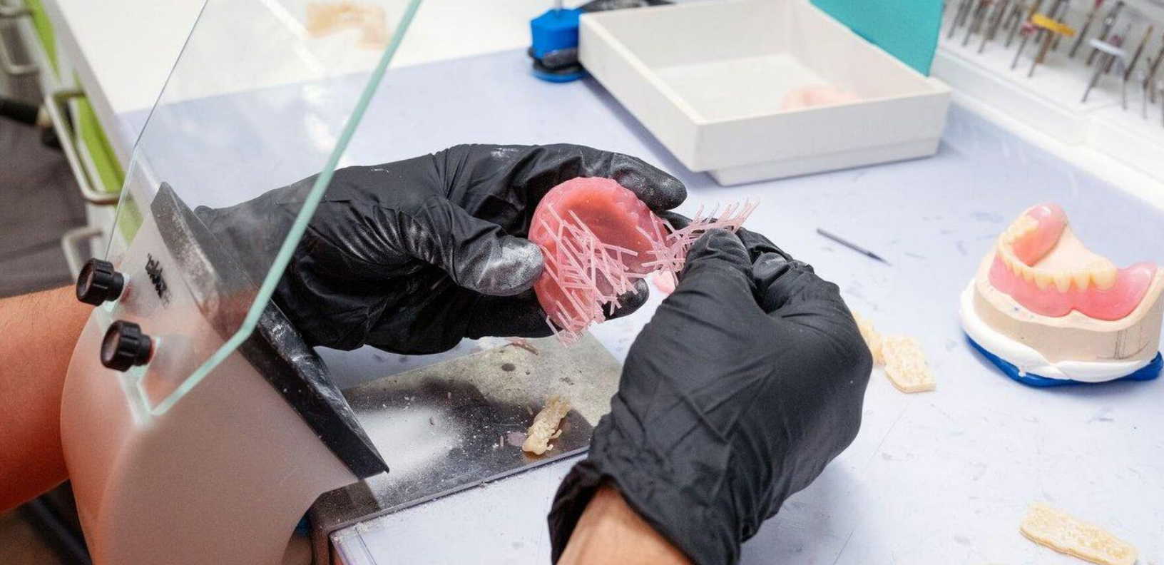
Easy removal of support structures from a denture base printed in Denture Base Resin.
