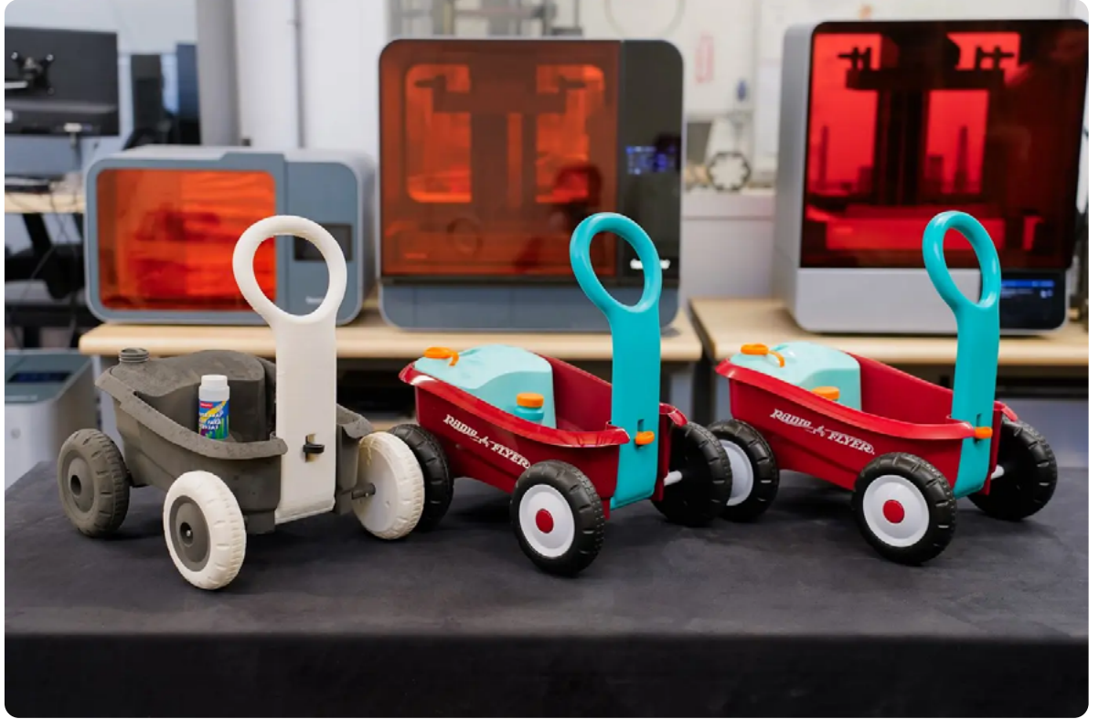
The original SLS printed prototype (left), SLA 3D printed and painted Roadshow Prototype (center) and final Production Bubble Buddy Walker Wagon .
