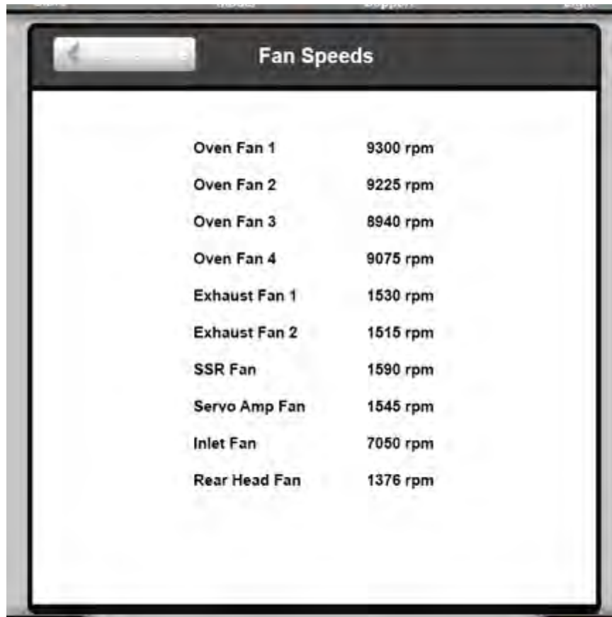
Figure 4-77: Fan Speeds Page - Fans Within Spec
