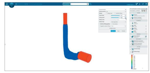
The flow path volume with normalized flow field selected and turned into geometry. (Picture courtesy of Dassault Systèmes.)
