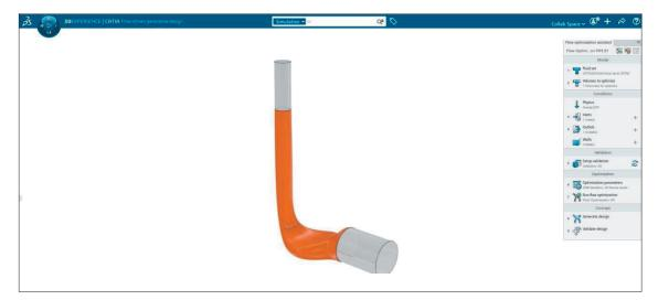
The rough volume of normal flow is automatically morphed into a smooth shape. (Picture courtesy of Dassault Systèmes.)
