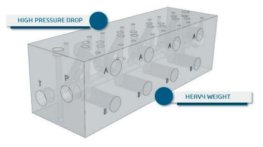
Hydraulic manifold legacy design has a high pressure drop from inlet to outlet and a mass of **8.3 Kg.** (Picture courtesy of Dassault Systèmes.)
