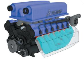
Internal flow optimization of an exhaust manifold. (Picture courtesy of Dassault Systèmes.)
