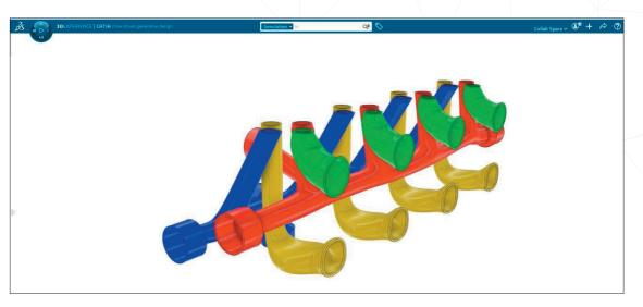
All smooth internal paths shown in hydraulic manifold. (Picture courtesy of Dassault Systèmes.)
