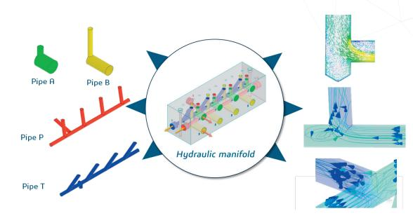
Hydraulic manifold showing internal fluid paths and valves. (Picture courtesy of Dassault Systèmes.)
