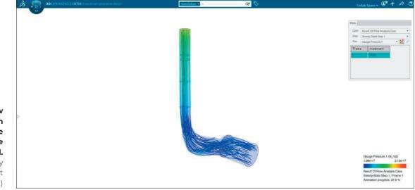
Flow lines show no recirculation in the volume cut out of the flow field. (Picture courtesy of Dassault Systèmes.)
