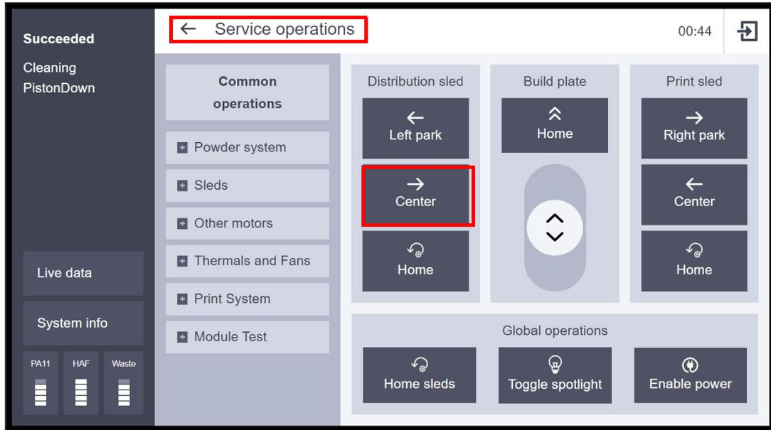
2. Once the distribution sled is moved to the center, press **Module Test | Sleds | Distribution sled**. See Figure 73.
