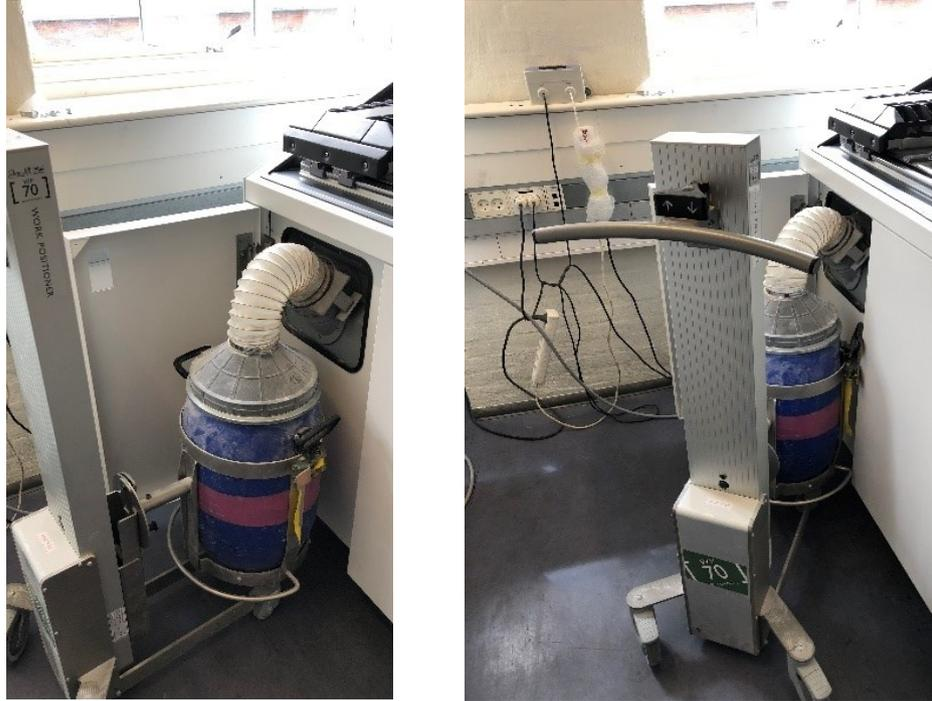
9. Begin raising the powder container. See Figure 20. The powder container will begin to tilt while it is being raised. Raise the container to the maximum height.
