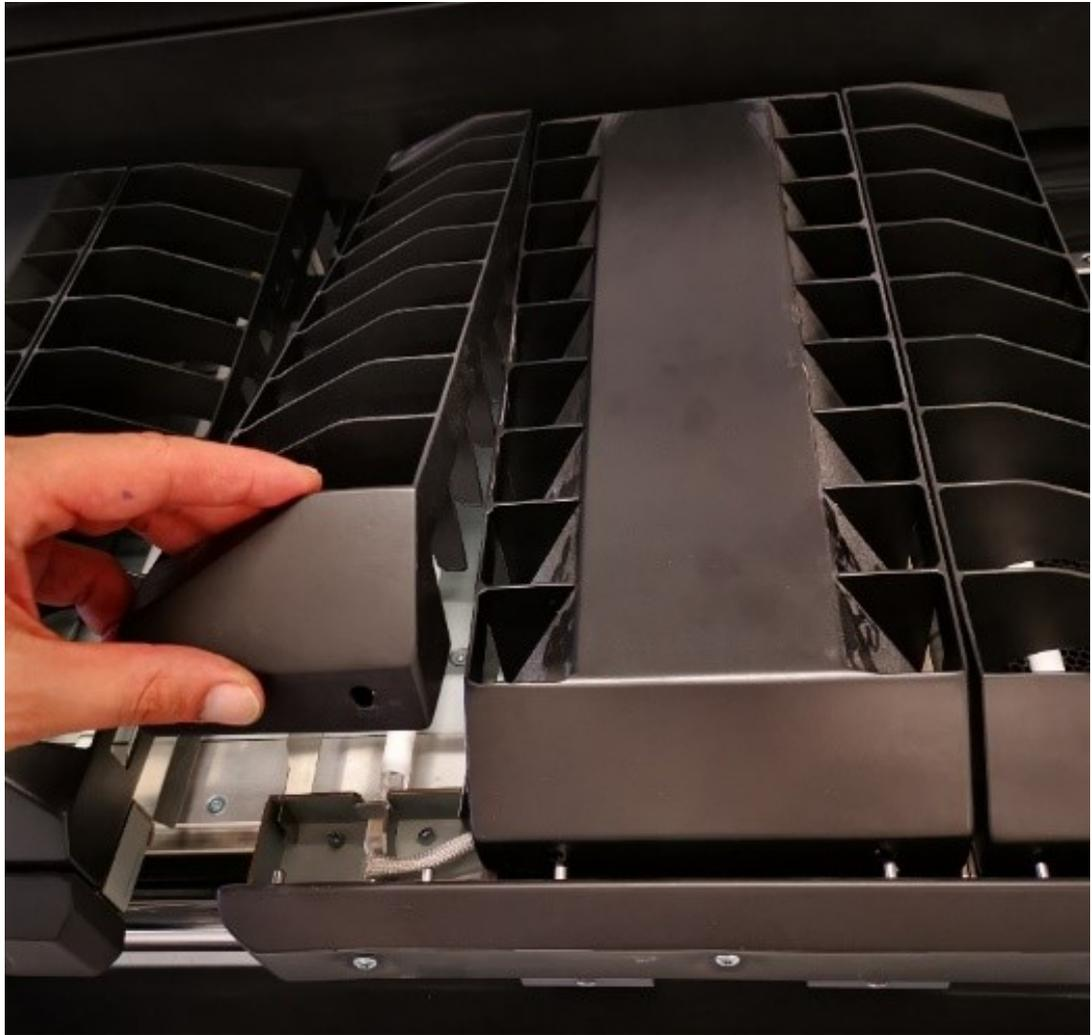
Figure 23: Distribution sled and Print sled with covers removed
