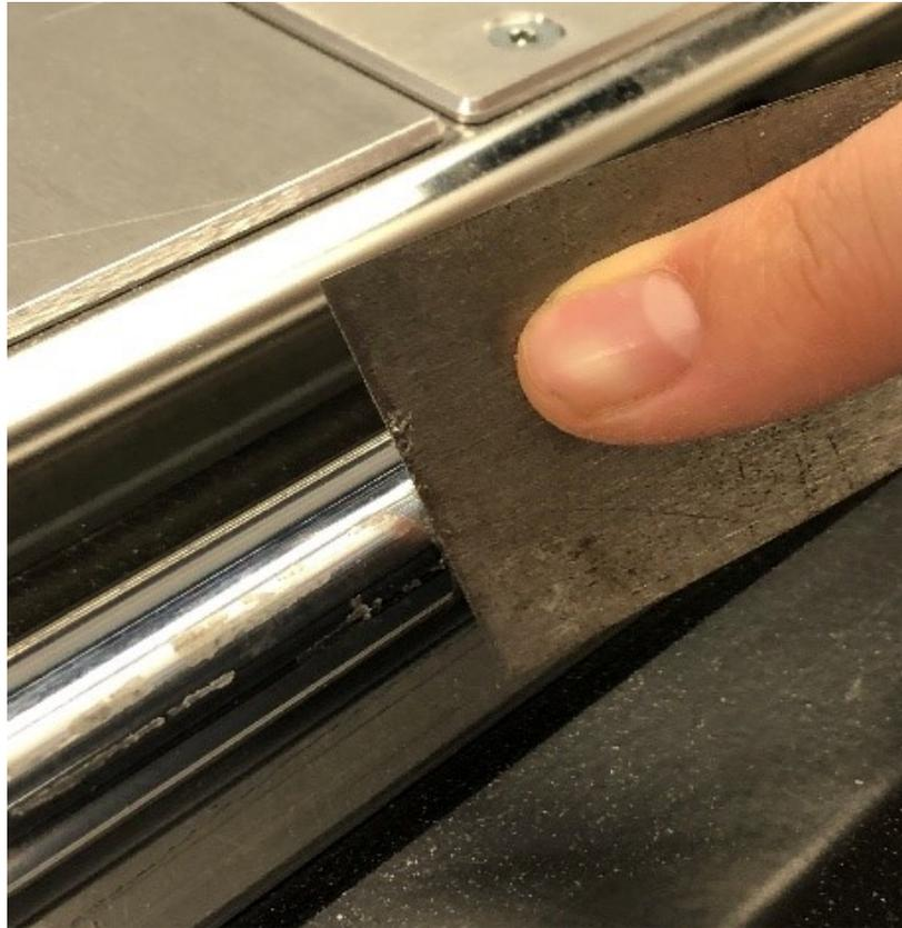
3. Scrape away the fused polymer from the guide surfaces. Move the sleds by hand to access the entire length of the guide. See Figure 83.
