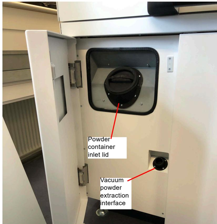
7. Mount the front end of the powder container adapter to the inlet of the printer.
