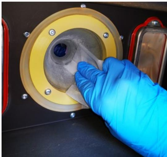
3. Once all soft particles have been removed, clean the thermal camera window with lint free pre-moistened towelettes. Use a gentle circular motion and apply very little pressure. See Figure 88.
