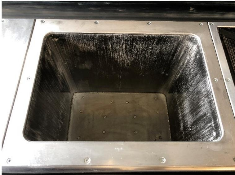
7. Vacuum the walls of the build chamber from excessive amounts of powder. See Figure 49.
