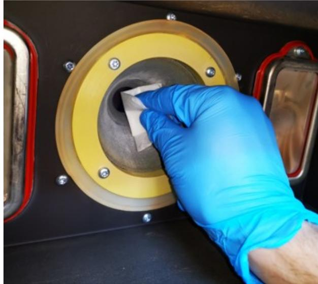
4. Before the liquid from the towelettes evaporates, use a swab to wipe the thermal window dry using a gentle circular motion and applying very little pressure. See Figure 89.
