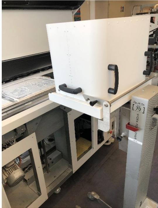
3. For safer transport of the build removal box, lower the Stratasys H-trolley tray.
