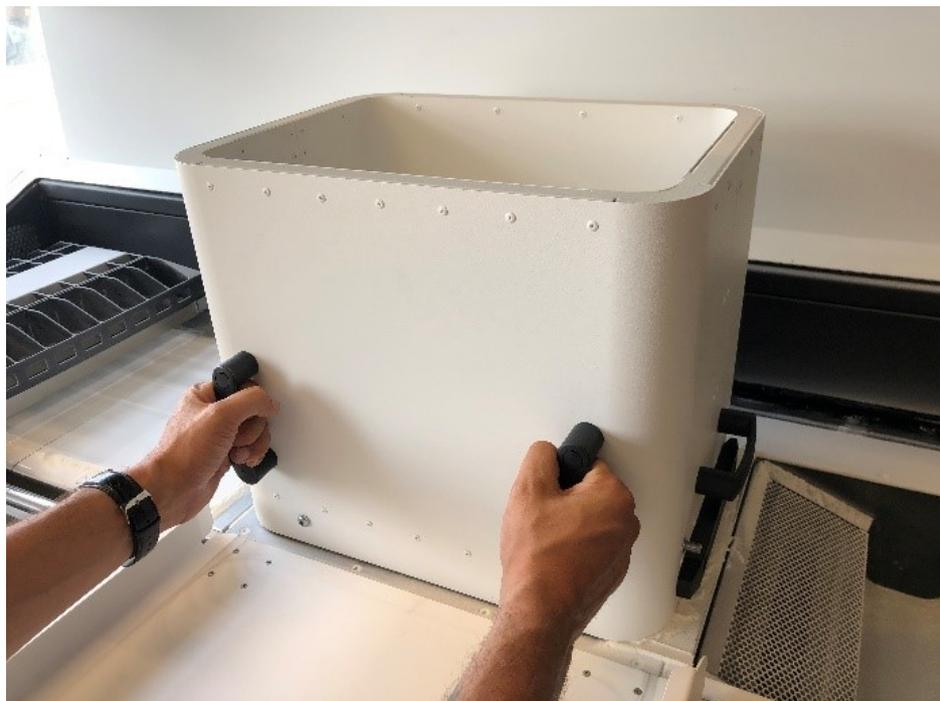
5. When the build removal box is properly positioned on the tray, engage the lock that secures the build removal box to the Stratasys H-trolley.
