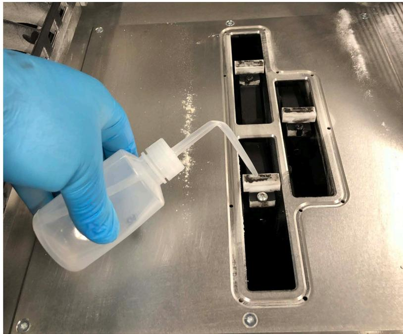
Figure 57: Cleaning the nozzles
