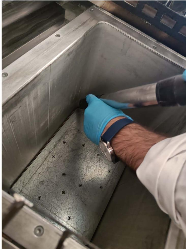
Figure 50: Cleaning the pinhead cleaning module
