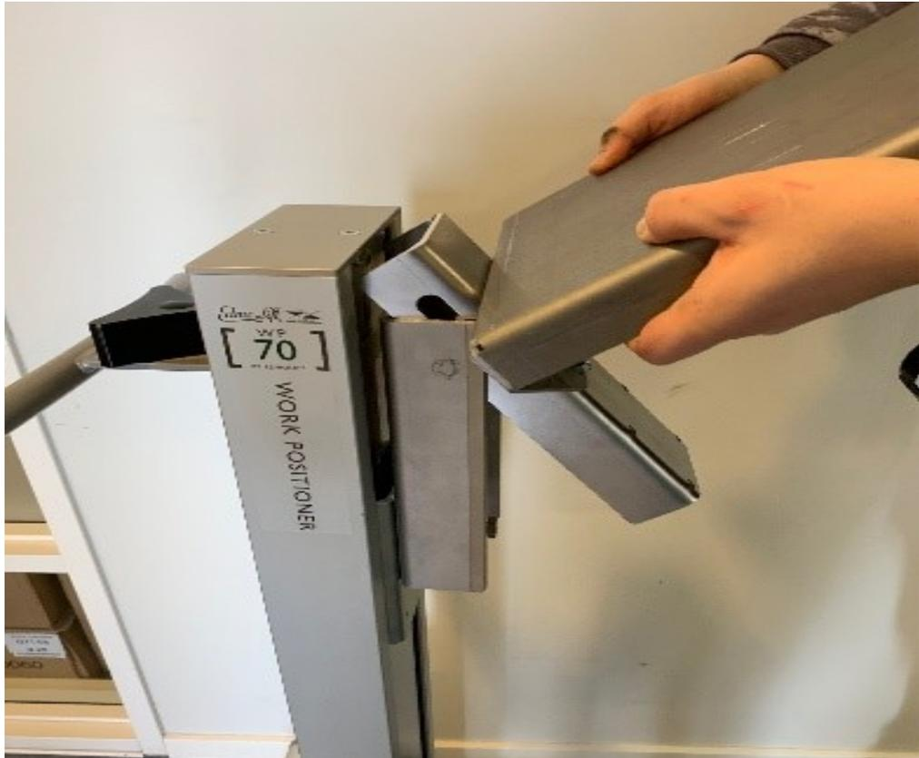
2. Confirm the bracket is locked properly in position using the lock pin. See Figure 36.
