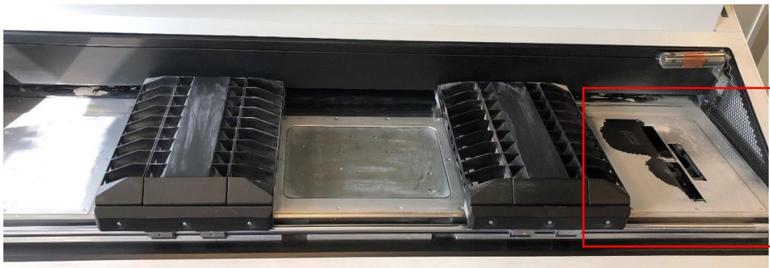
8. In some cases, there will be dried fluid under the parked print sled. Use a wet wipe to remove the dry fluid. See [Figure 51](#). Wipe the surface with dry paper towel in order to avoid powder sticking to the wet surface.
