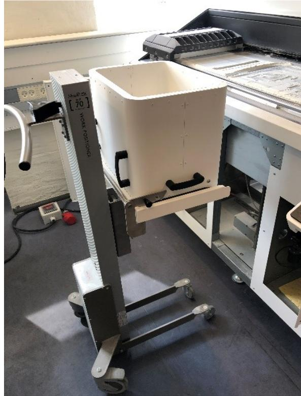
**i** The Stratasys H-trolley can safely and stably carry the build removal box even when fully extended.
