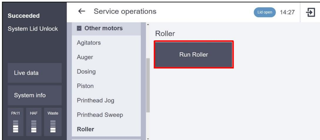
**i** If excessive resistance is applied to the spinning roller, the roller will stop. Press **Run roller** to restart the roller and continue the cleaning process.
