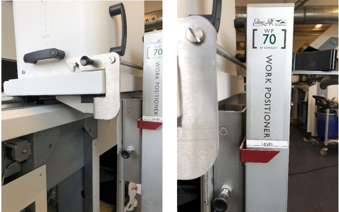
6. If the build removal box is not level, the markers will appear as shown below. See Figure 44.
