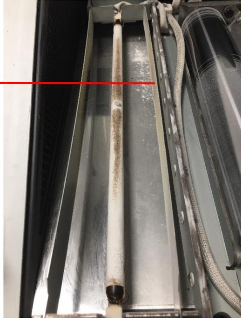
2. When the strip is removed, clean the distribution sled surface of all powder.
