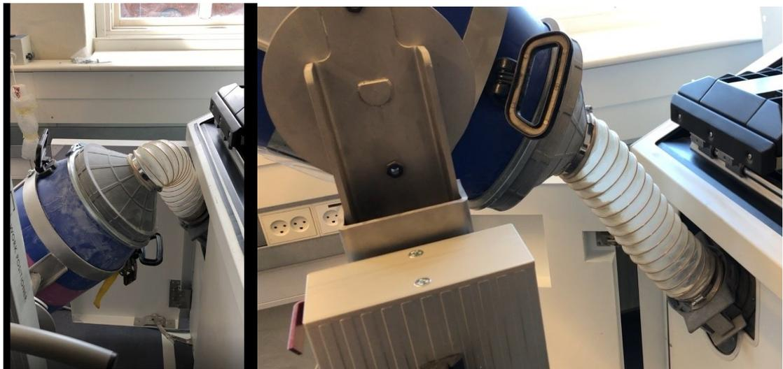
10. Raise the powder container to its maximum height. Lock the powder container so it will remain inverted vertically. See Figure 21. The powder will start flowing from the powder container into the printer.
