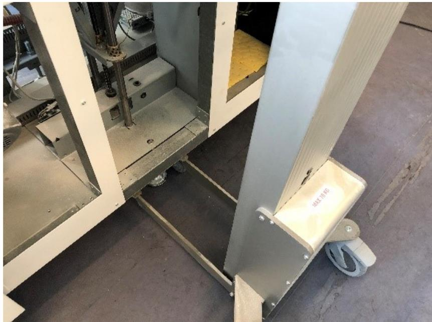
Figure 41: Build removal box lifted above the level of the printer top plate
