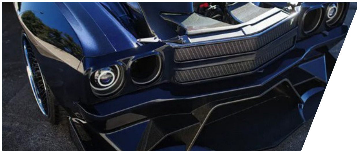
Blazin Rodz Doughboy front bumper - 3D printed with HP MJF
