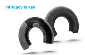
The Ink Hose Flow Bend Clip, routes ink hoses in and out of printheads. The purpose of this part is to prevent the hose from kinking while maintaining a sharp bend. Although this is a standard industrial concept, the part was customized so it could accommodate the required angle in the limited space. This intricacy was achieved on the H350 through exact design specifications and the ability to print precisely.
