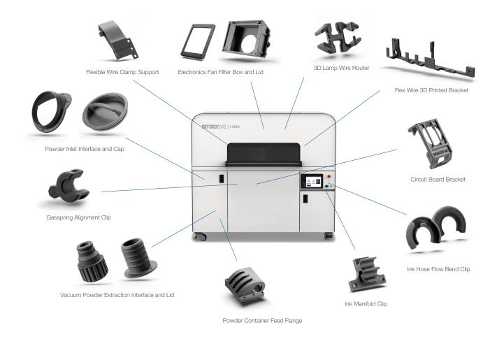
Printing with the H350 enabled a faster time to market and saved unnecessary production and transportation fees. As compared to days or even weeks with traditional manufacturing, accurate enduse parts for the H350 were produced and ready for implementation within hours.
