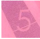
Figure 4-52 Missing line in the test print
