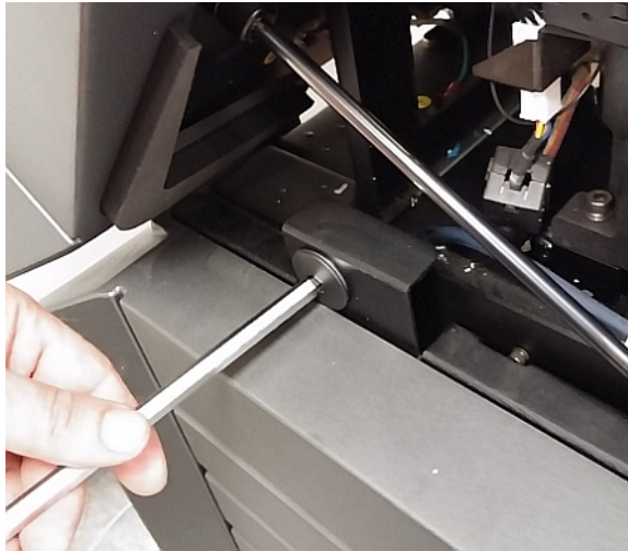
Figure 4-110 Opening a panel latch
