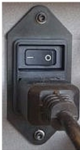
Figure 4-2 Main power switch and cable
