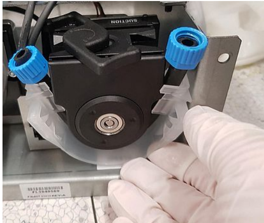
Figure 4-143 Installing the new tube
