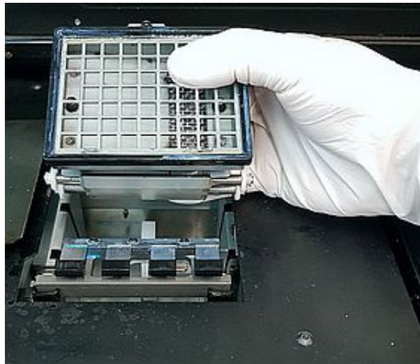
Figure 4-47 Removing the purge unit waste collector
