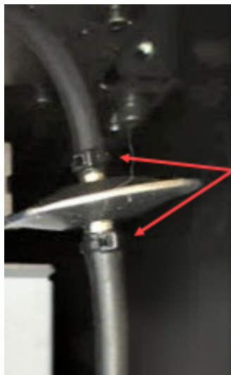
Figure 4-171 Material filters tie wraps
