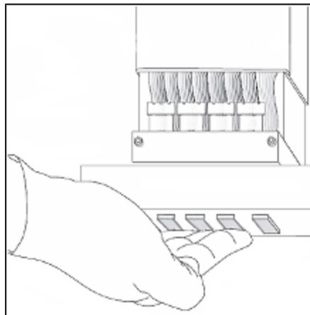
Figure 4-126 Checking the level of the new head
