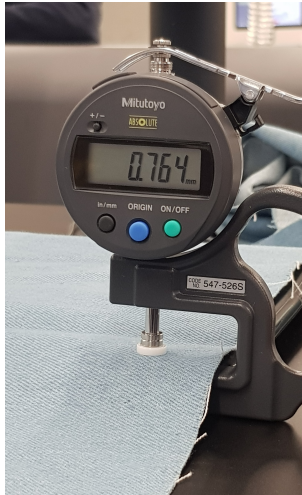
Figure 4-10 Measuring the fabric thickness
