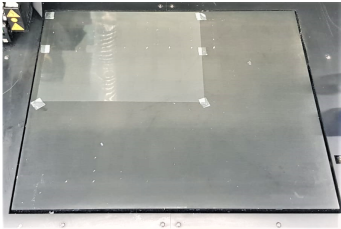
Figure 4-195 Fixing the transparency to the tray
