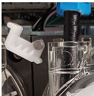
Figure 4-163 Releasing the pump (sample)
