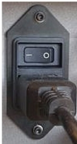
Figure 4-2 Main power switch and cable
