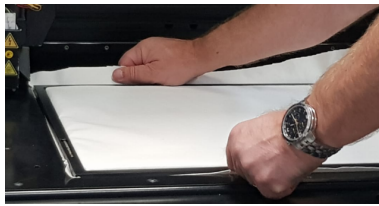
Figure 4-20 Stretching the fabric on the non-elevated tray (sample)
