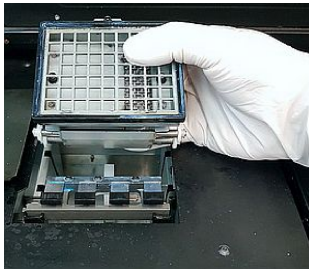
Figure 4-71 Removing the purge unit waste collector
