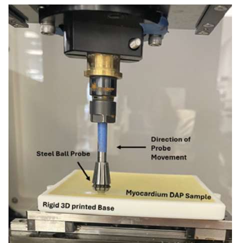
Figure 3- Lubricity test fixturing showing the printed myocardium sample loaded into the rigid 3D printed test fixture. The rod travels from the middle of the sample to the left for each iteration.
