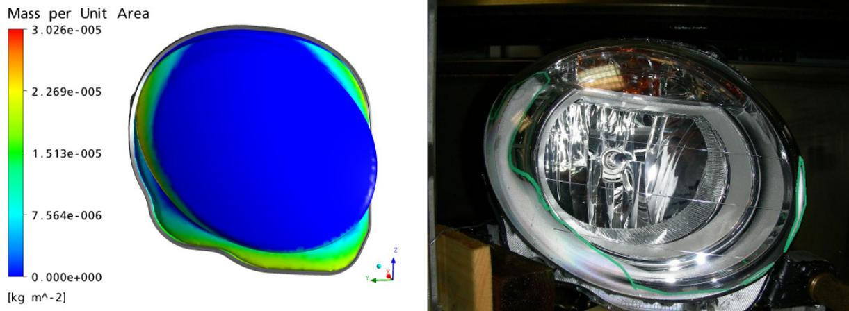
Figure 10: qualitative comparison between numerical and experimental results
