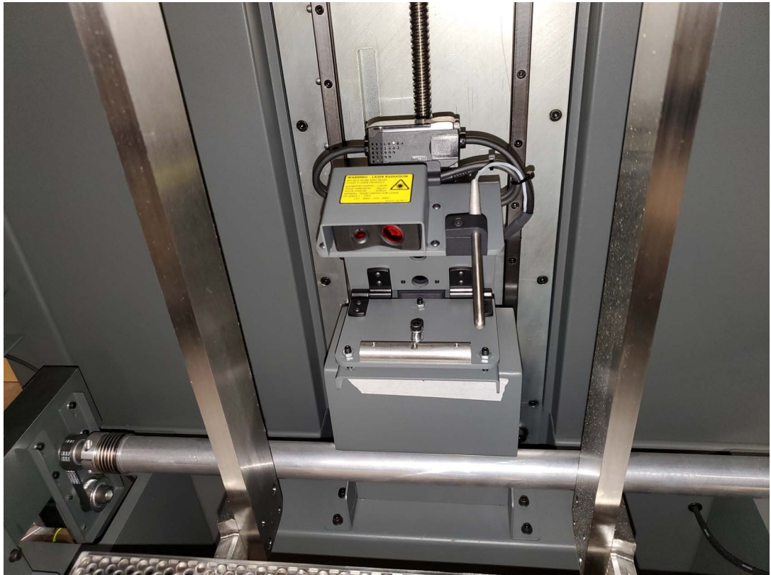
Figure 31: Neo450 resin leveling sensor, rotated up
