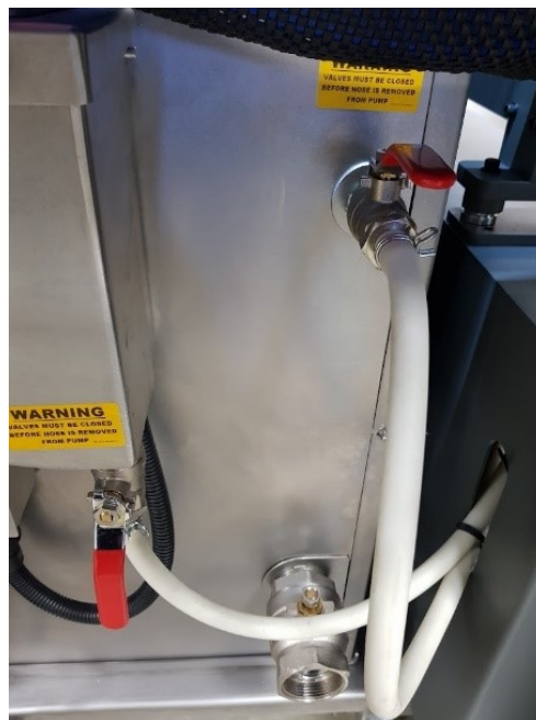
Figure 11: Neo450 Peristaltic resin pump and tubing installed
