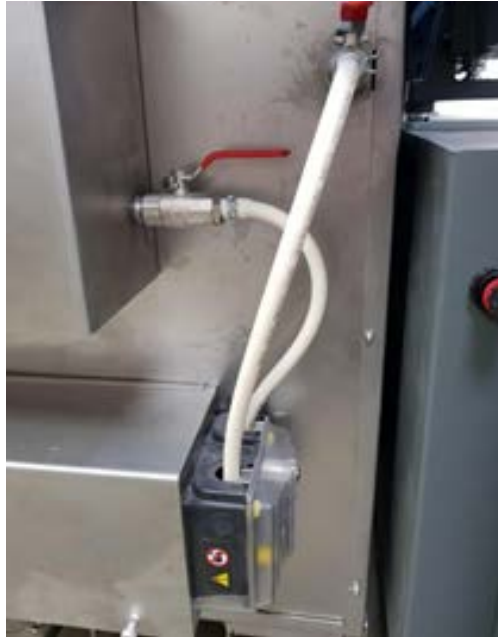
Figure 11: Neo450 Peristaltic resin pump and tubing installed
