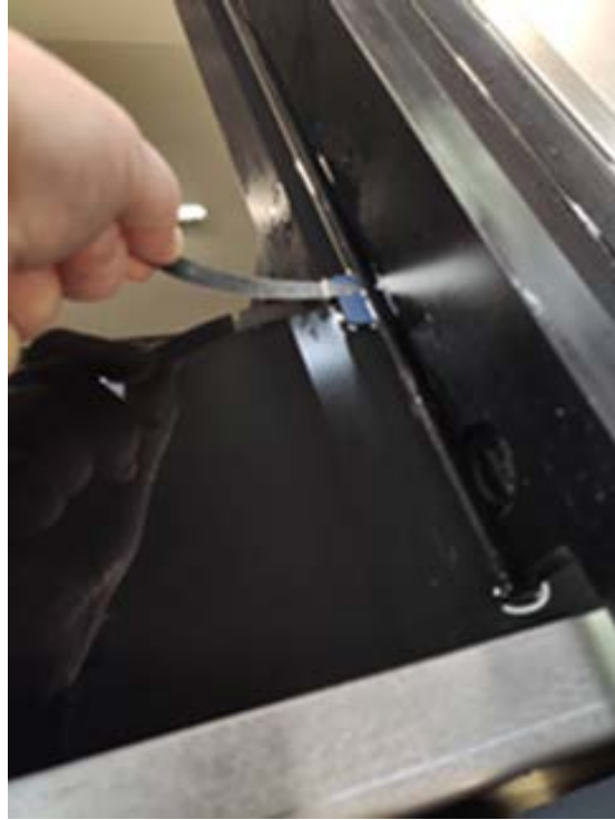
Figure 20: Recoater blade height adjustment and locking bolts
