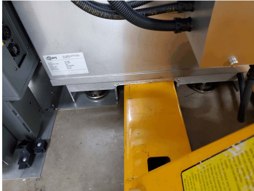
Figure 218: Lifting the vat
