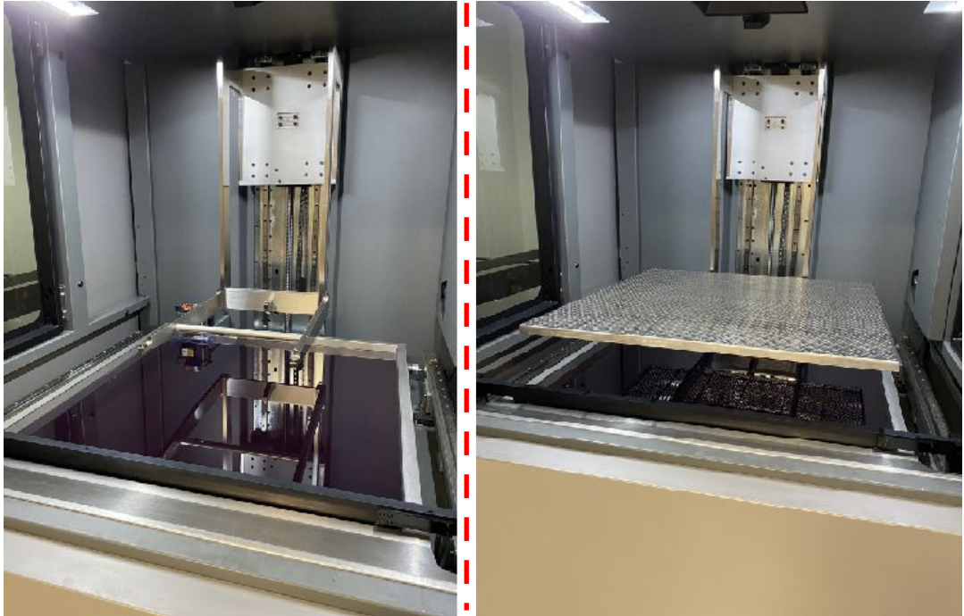
Figure 177: Installing the build platform
