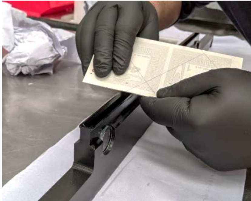
Figure 239: Removing resin deposits
