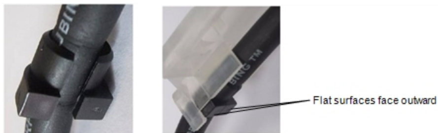
Figure 6-94 Left: Tube clamps; Right: Tube inserted into tube holders
