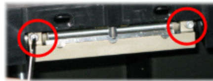
Figure 6-44 Removing the roller waste collector
