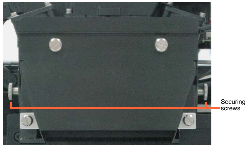
Figure 6-41: UV-lamp-assembly securing screws
