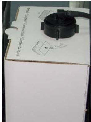
Figure 6-71: Waste container with drain tube attached
