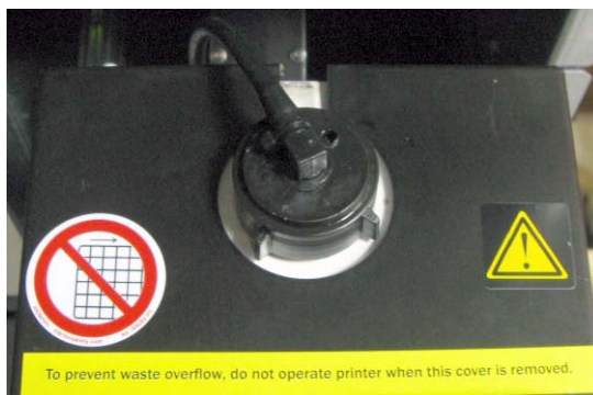
Figure 6-72: Fireproof cover installed over the waste container
