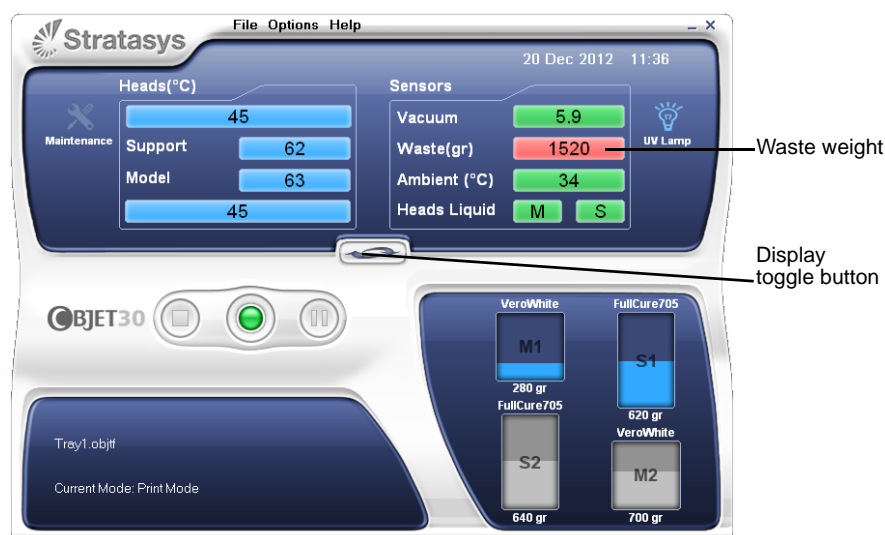
Figure 6-69: Printer interface, showing waste weight (red background indicates operator alert)
