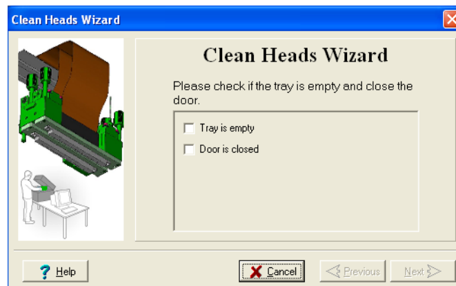
Figure 6-27: Head cleaning procedure—wizard screen
