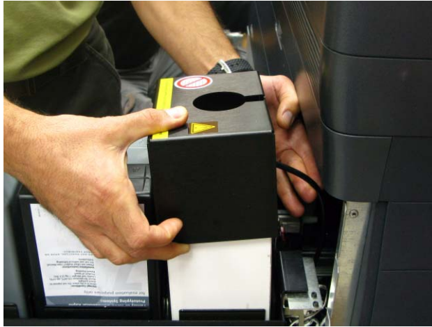
Figure 6-70: Removing the waste-container cover
