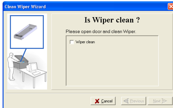
Figure 6-36: Wiper Cleaning Wizard during steps 7–10
