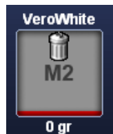
Figure 6-6: Empty cartridge indicator
