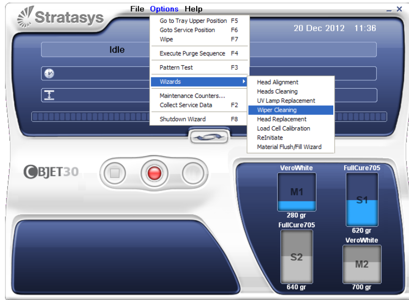
Figure 6-34: Starting the Wiper Cleaning Wizard
