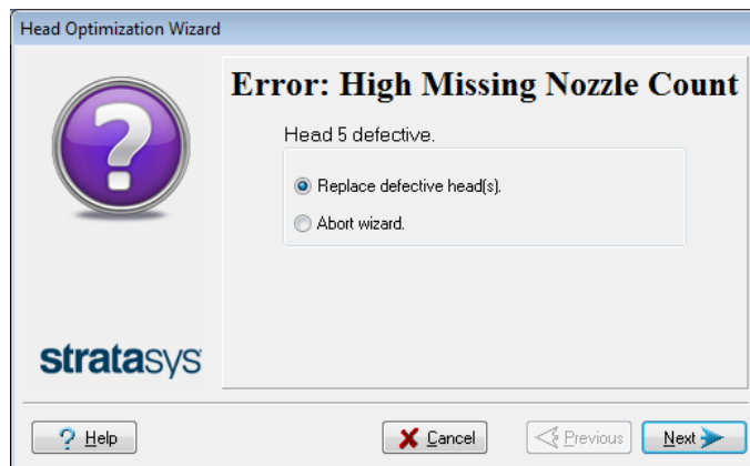
Figure 6-65 Head replacement due to missing nozzles
