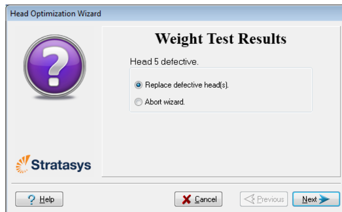
Figure 6-70 Defective print heads found
