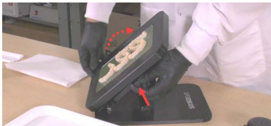
Figure 19: Pulling pin for rotating part removal jig
