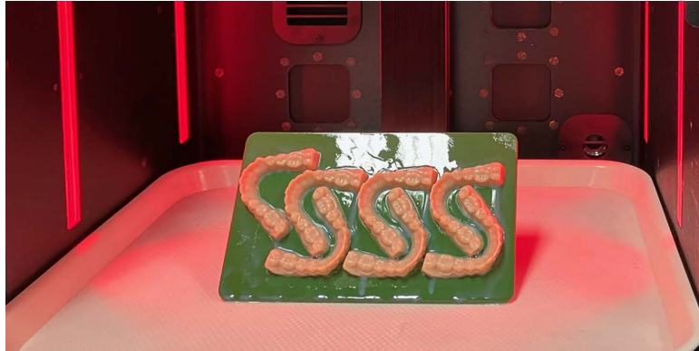
Figure 17: Build platform placed on the tray
