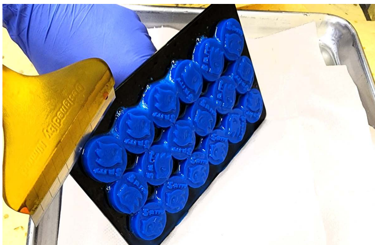
Figure 10: Holding the build platform and scraper—cut-resistant glove is under the nitrile glove on the non-dominant hand
