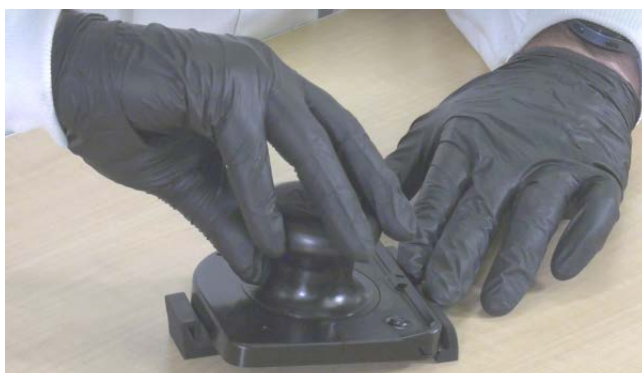
Figure 25: Placing scraper jig into scraper holding jig
