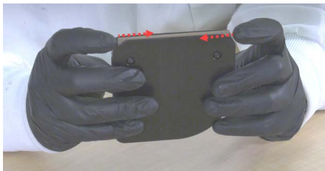
Figure 23: Centering blade horizontally
