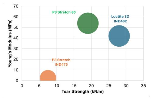
Higher Young's Modulus values indicate that the material is stiffer and has a higher Shore Hardness value. Elastomers with higher stiffness are generally more resistant to tearing.
