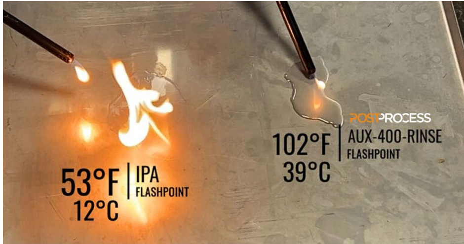
Figure 3: IPA Ignited next to AUX-400-RINSE which will not ignite
