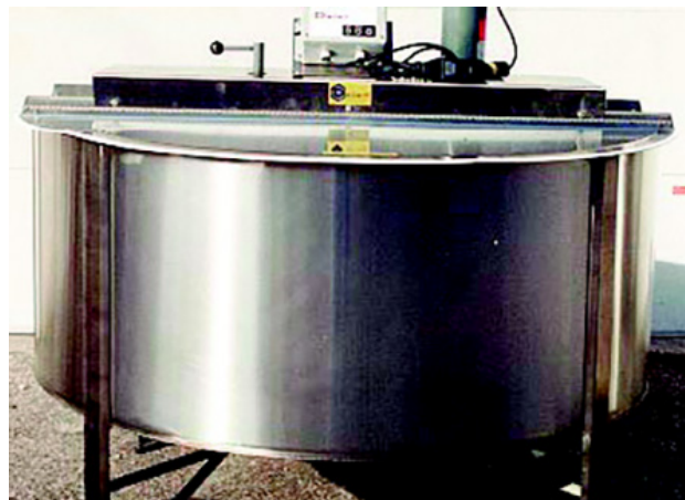
Honey spinner used for removing resin from the pattern
