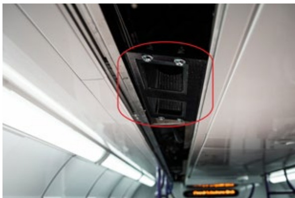
A view of the 3D printed vent located in the train cabin ceiling (circled).
