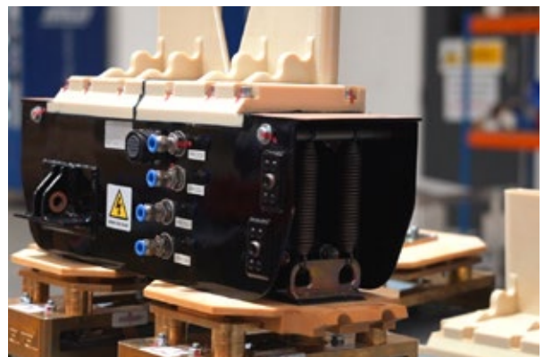
A view of the ULTEM™ 9085 resin parts installed on top of the fast-charge shoe gear system.
