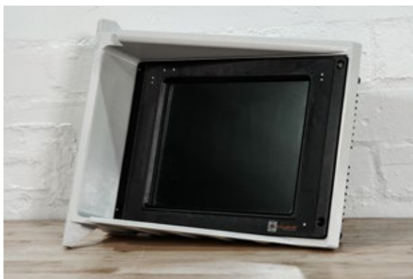
The 3D printed bezel made with Kimya PC-FR material surrounding the driver's display panel.
