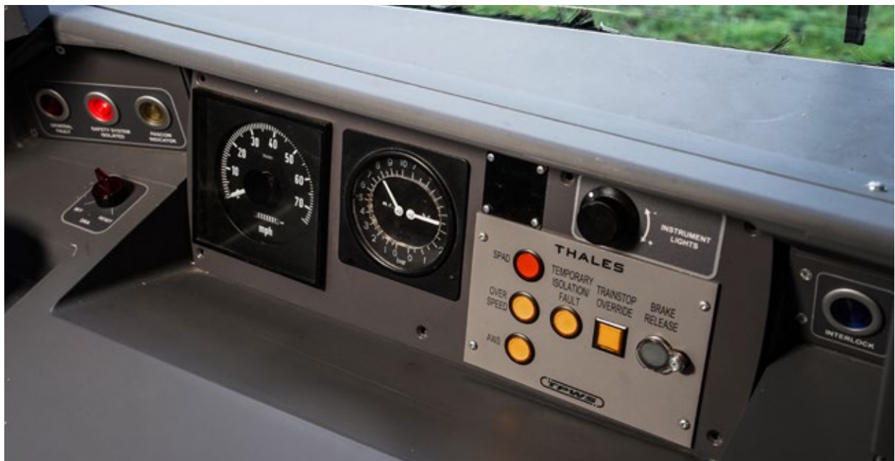
The 3D printed dash assembly installed in the train.
