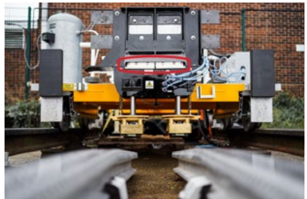
The test bed for the fast-charge system showing the location of the 3D printed ULTEM™ parts (circled).
