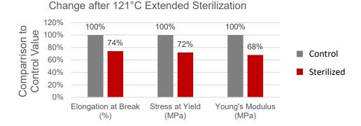
**Ethylene Oxide (EtO) Sterilization**
