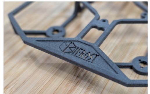
A close-up of the printed frame showing some of the detail achievable with SAF technology.
