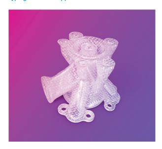
Waiting weeks for metal tooling is no longer needed with 3D printing. Specialized equipment and tooling costs for wax pattern production are also eliminated. Complex and intricate patterns are possible so engineers can optimize the cast for the part rather than for the mold-making process. And the ability to quickly print and test multiple design variations is easier to accomplish compared with traditional manufacturing.
