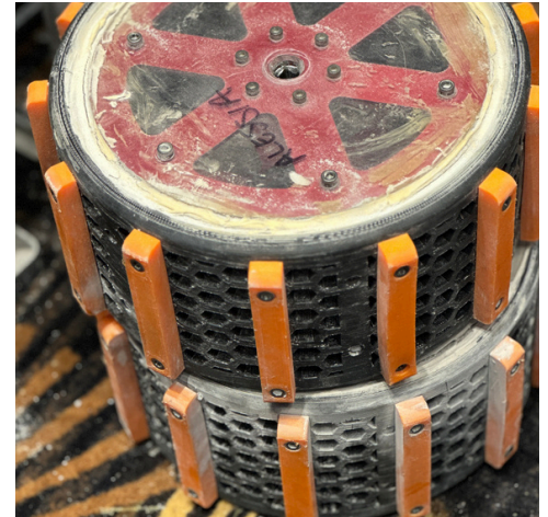
Wheel assembly made using FDM TPU 92A
