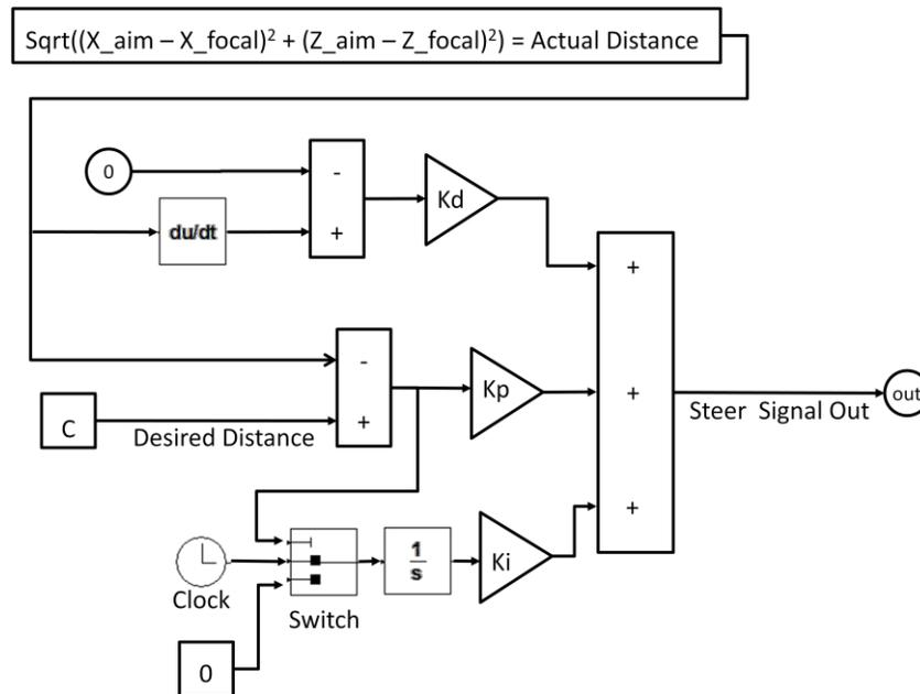
Figure vi - Steady State Turning Circle Steer Command
