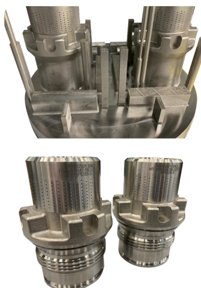
Image 4a & b. (a. Top) Two choke valves, optimized with IMI's DRAG technology, shown on the build plate after being 3D printed with Velo3D's Sapphire® system, and (b. Bottom) the two valves after finishing.
