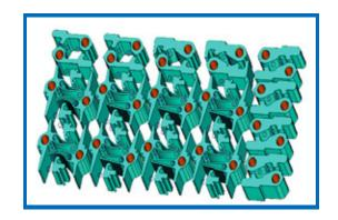
CAMWorks Wire EDM Pro includes automatic programming for complex 2-axis, 2-axis with taper and full 4-axis wire EDM machining.
